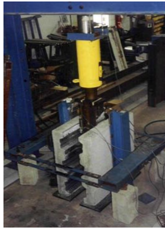
Figure 22 Push-out Testing Setup at Virginia Tech
