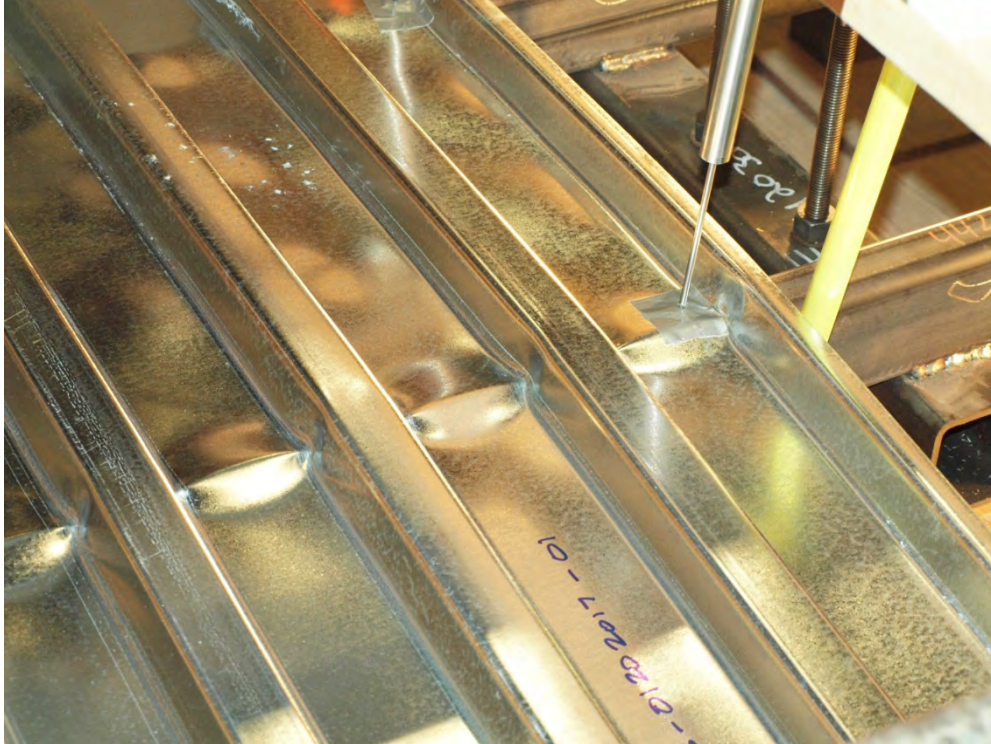
Figure 61: 20 Gage Deck Positive Bending - Further Buckling.
