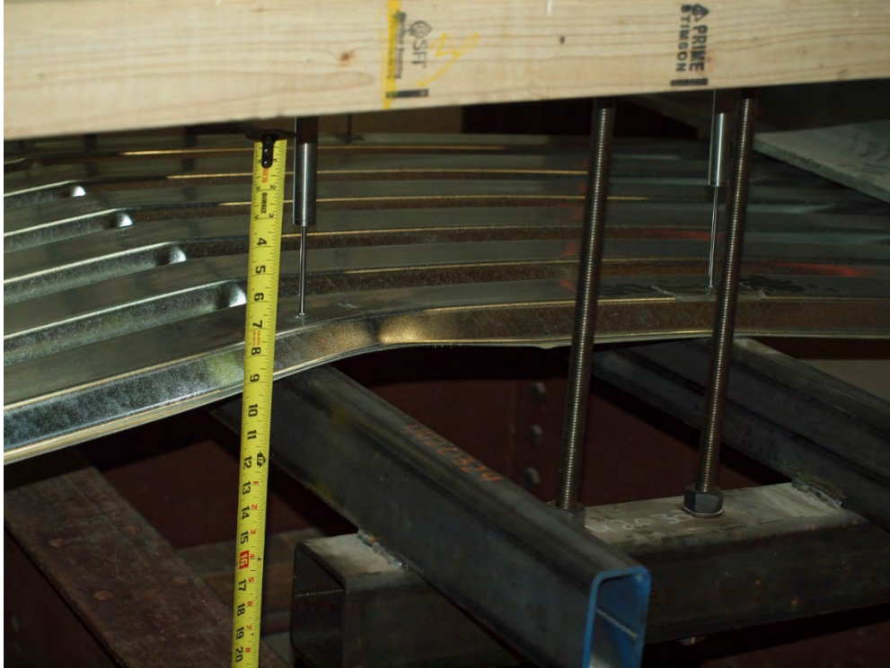
Figure 24: 16 Gage Deck Negative Bending - Final State.
