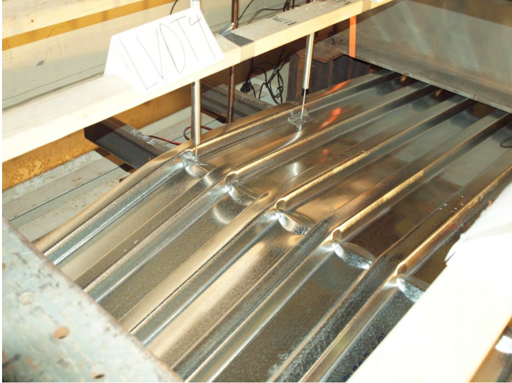
Figure 62: 20 Gage Deck Positive Bending - Final State.
