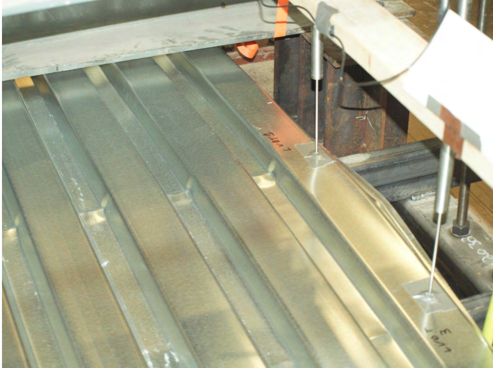
Figure 67: 22 Gage Deck Negative Bending - Initial Buckling.
