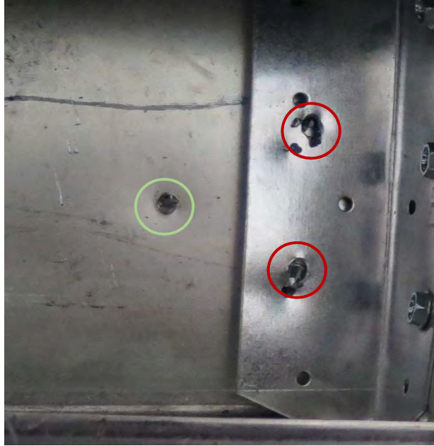
Figure 3.5 Shear failure of screws: shear capacity conserved on all the layers (in green) and capacity lost on the top layer (in red)
