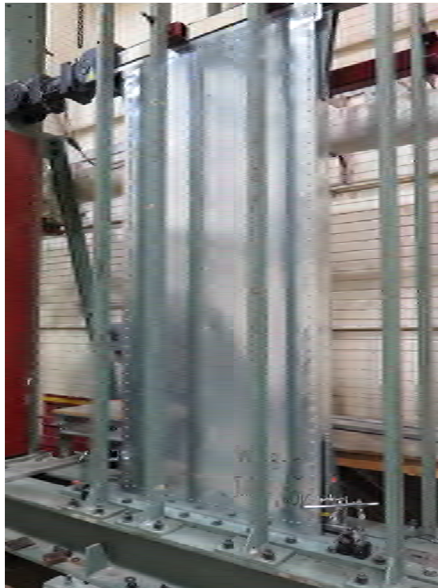
Figure 2.15 Double-sheathed configuration: specimen ready to be tested
