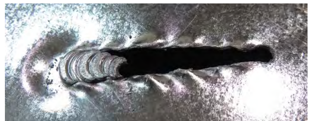
Figure 3.2 Steel bearing damage in sheathing from centre-sheathed configuration
