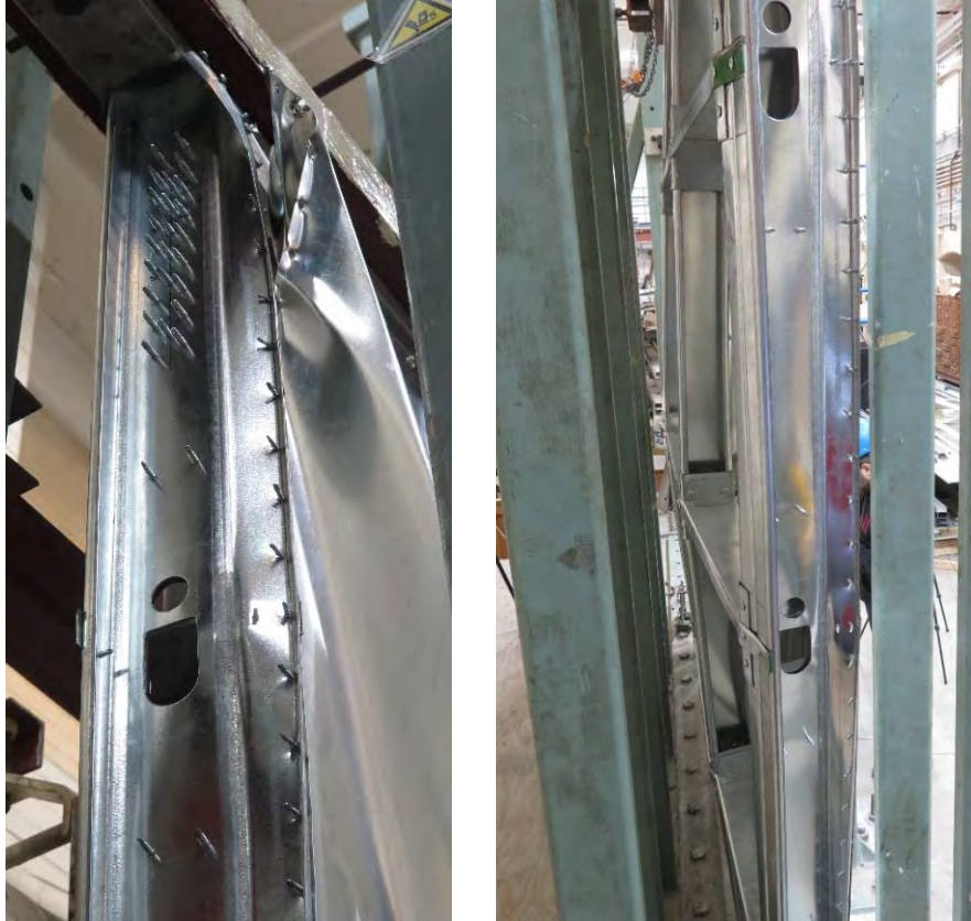
Figure 2.1. Damage due to eccentric sheathing placement: a. torsional forces on chord stud, and b. out-of-plane forces on centre stud due to shear buckling of the sheathing (Rizk (2017))
