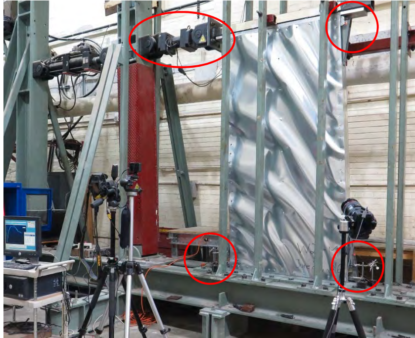
Figure 2.25: Placement of test instrumentation. Loadcell shown at the top left, string potentiometer at the top right, and LVDTs at the bottom.
