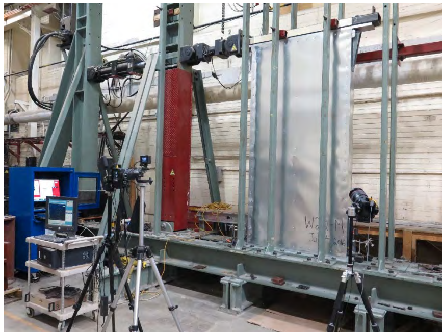
Figure 2.2: Shear wall specimen installed in test frame.
