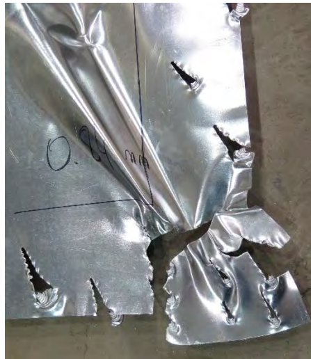
Figure 3.6: Bottom corner tear-out sheathing failure of centre-sheathed specimen W25-CR3.
