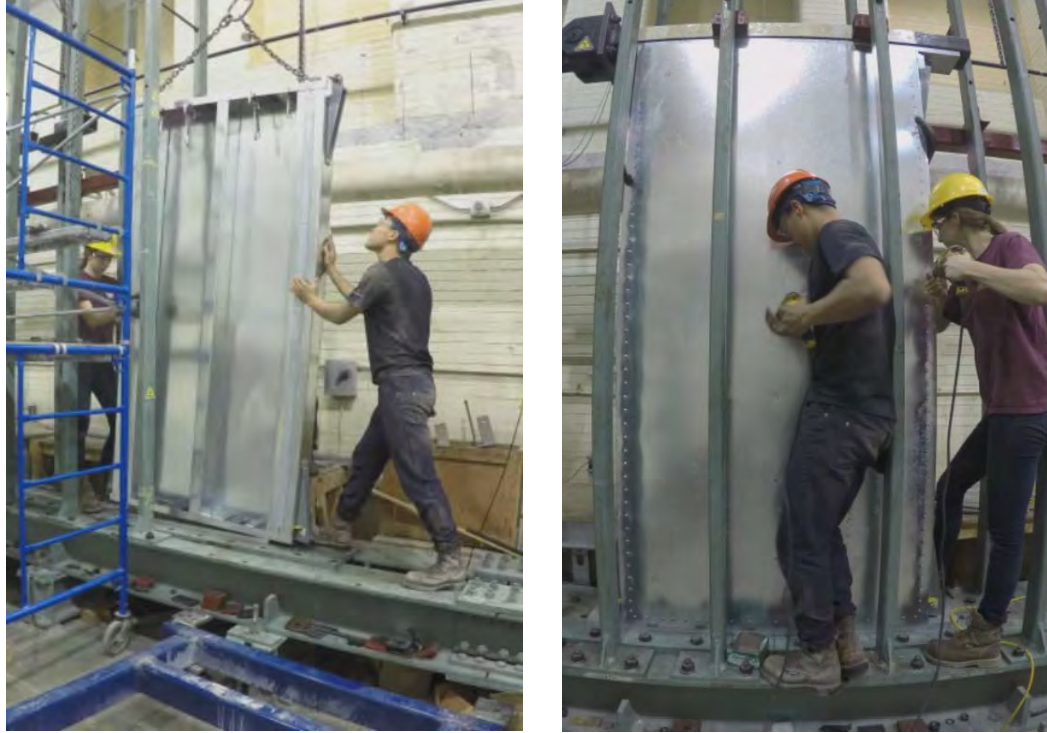
Figure 2.15: A) Installation of specimen into the testing frame. B) Installation of second sheathing panel.
