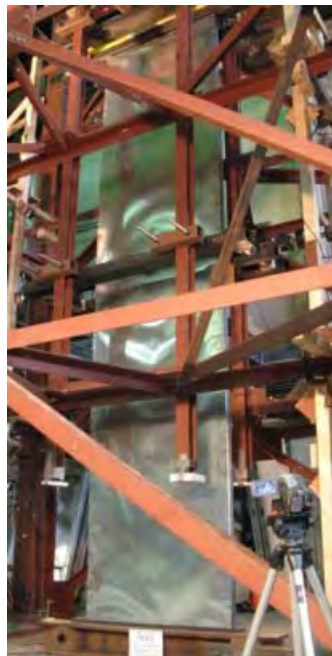
Figure 1.6: Steel sheathed wall specimen on the shake table (Shamim (2012)).
