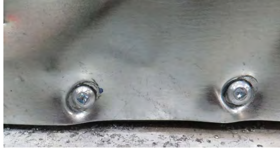
Figure 2.13 Sheathing steel bearing
