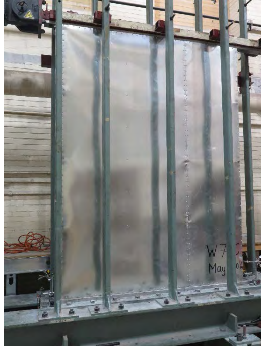
Figure 2.7 Sheathing combination for 1830×2440 mm (6'×8') shear walls
