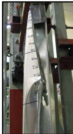
Figure 1.6 Chord twisting of unblocked walls (Balh, 2010)
