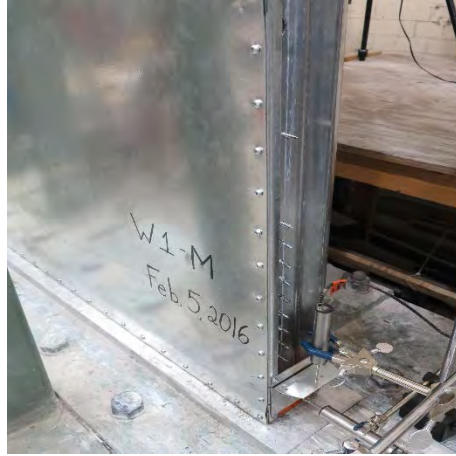
Figure 2.9 LVDT placement on non-structural steel plate
