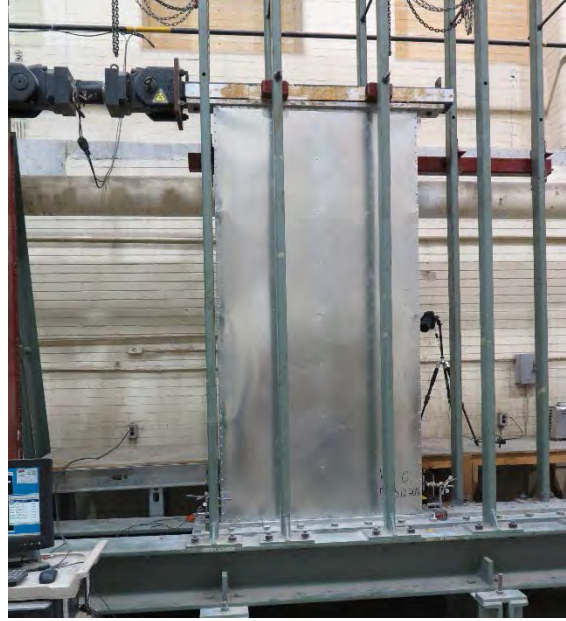
Figure 2.2 Typical wall installation in test frame
