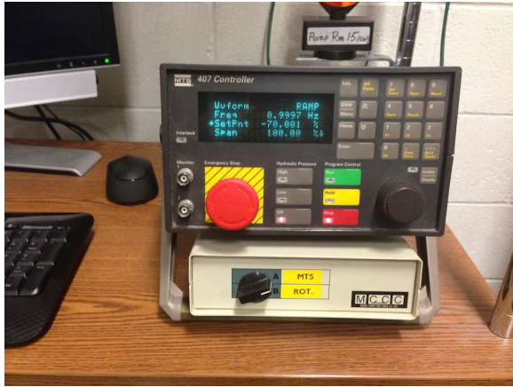
(a) MTS 407 controller
