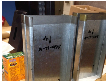
(b) Stripped zinc-coating
