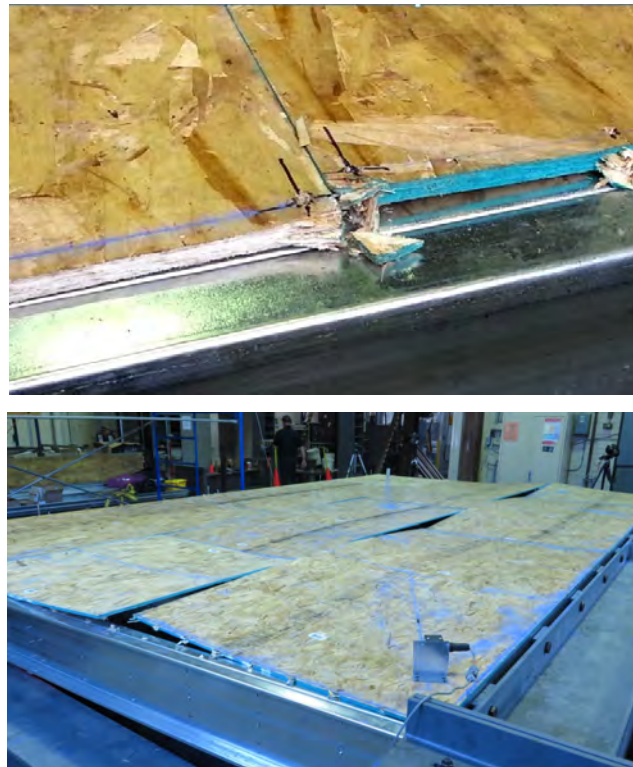
(b) Deformation from cyclic loading
