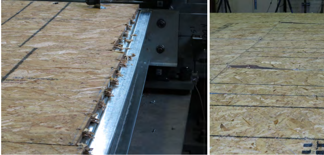
(b) Diaphragm behaviour from cyclic loading
