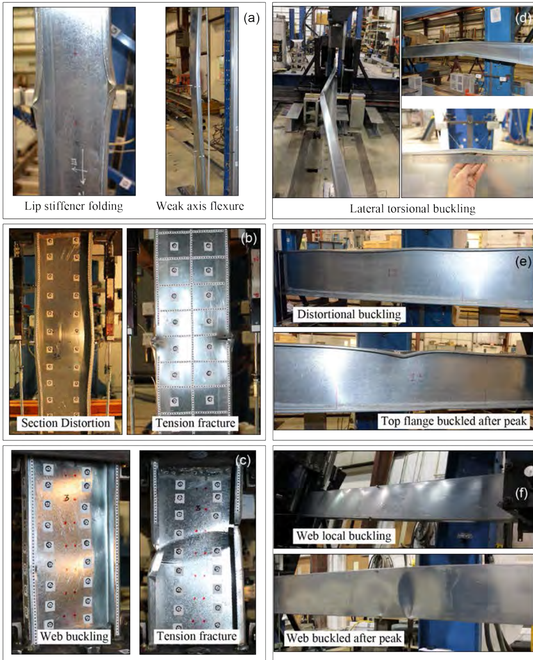
Fig. 1.2. Cold-formed steel member failure modes: (a) global buckling in axial member; (b) distortional buckling in axial member; (c) local buckling in axial member; (d) global buckling in flexural member; (e) distortional buckling in flexural members; (f) local buckling.
