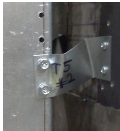
Figure 2.4: Test result of clip angle T5a #2
