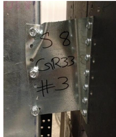
Figure 2.5: Test result of clip angle S8 #3
