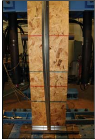
(c) torsion (T) in stud, typical for bare or one-sided sheathing cases, BO case shown
