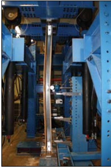
(a) local buckling (L) limit state in OG specimen, similar for OO specimens
