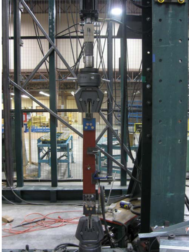
Fig 3.3 Setup #2 for Tension Tests on Bolted Connections
