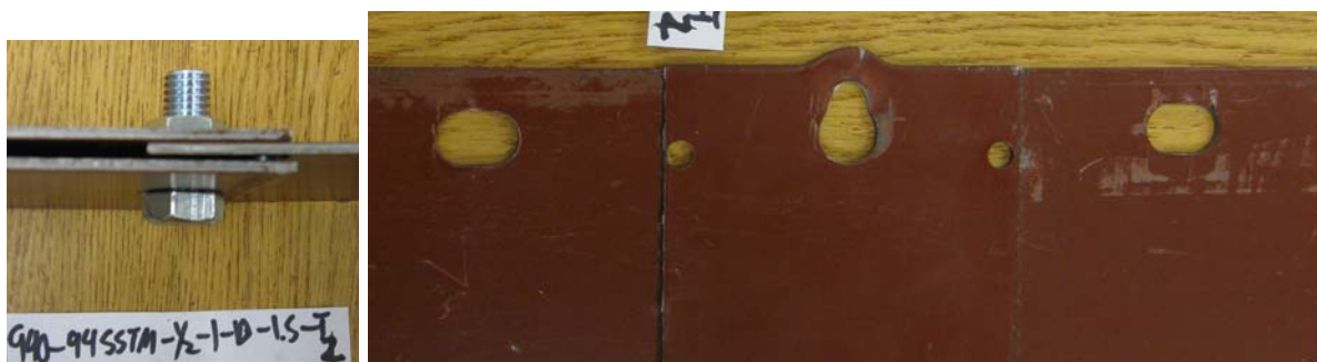
Fig 5.35 Shear Failure of Test Specimen 94O-94SSTM-1/2-1-D-1.5-T2
