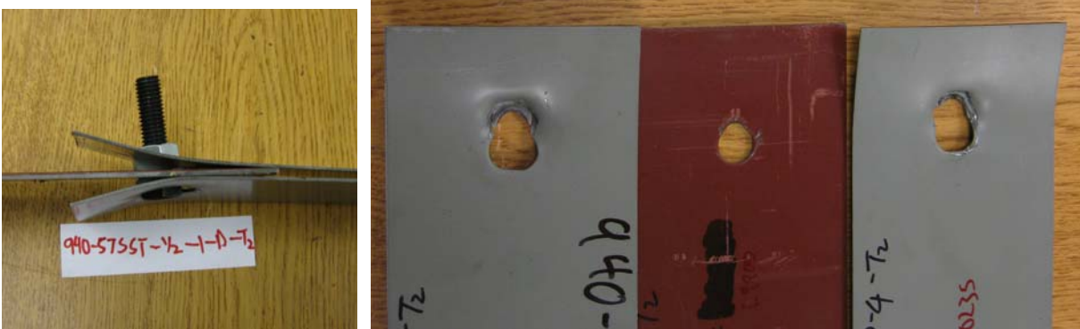
Fig 5.17 Bearing Failure of Test Specimen 940-57SST-1/2-1-D-4-T2
