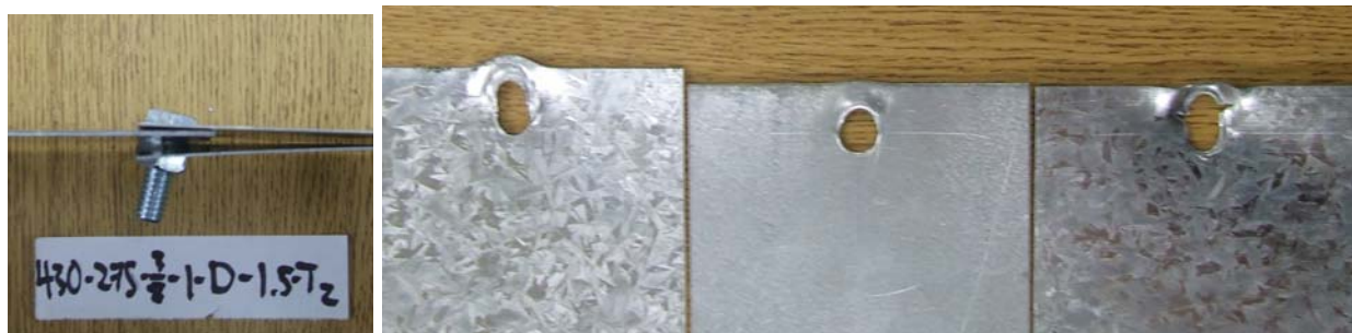
Fig 5.27 Shear Failure of Test Specimen 430-27S-3/8-1-D-1.5-T2
