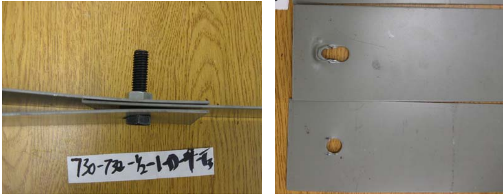
Fig 5.7 Bearing Failure of Test Specimen 730-730-1/2-1-D-4-T3
