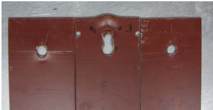
Fig 5.11 Bearing Failure of Test Specimen 94O-94S-1/2-1-D-4-T2
