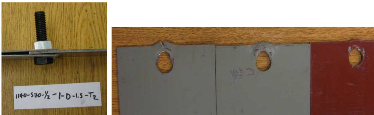
Fig 5.22 Shear Failure of Test Specimen 1140-570-1/2-1-D-1.5-T2
