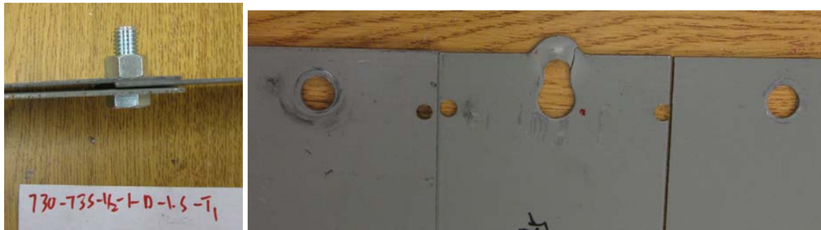
Fig 5.26 Shear Failure of Test Specimen 730-73S-1/2-1-D-1.5-T1
