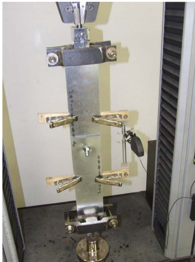
Fig 3.1 Setup #1 for Tension Tests on Bolted Connections
