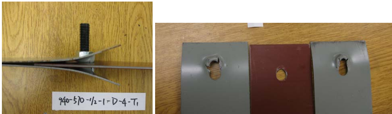
Fig 5.4 Sheet Bearing Failure of Test Specimen 940-570-1/2-1-D-4-T1
