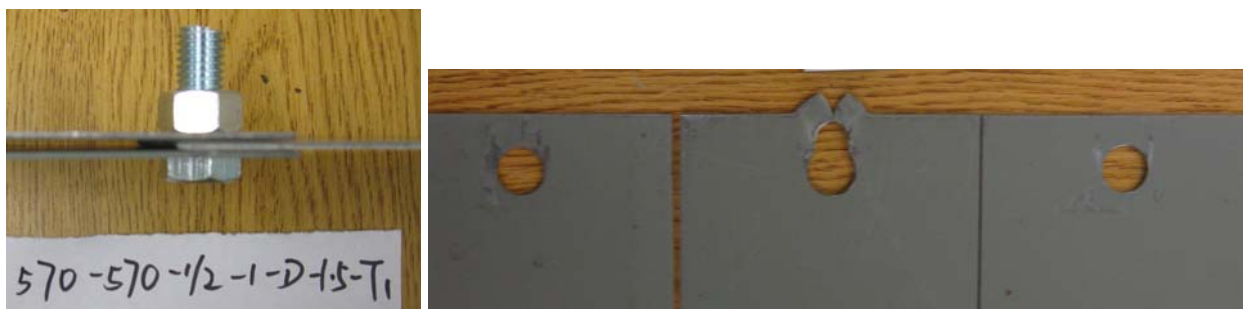
Fig 5.20 Shear Failure of Test Specimen 570-570-1/2-1-D-1.5-T1
