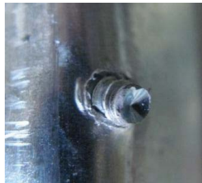
Figure 2.19 Screw Shear Fracture Failure
