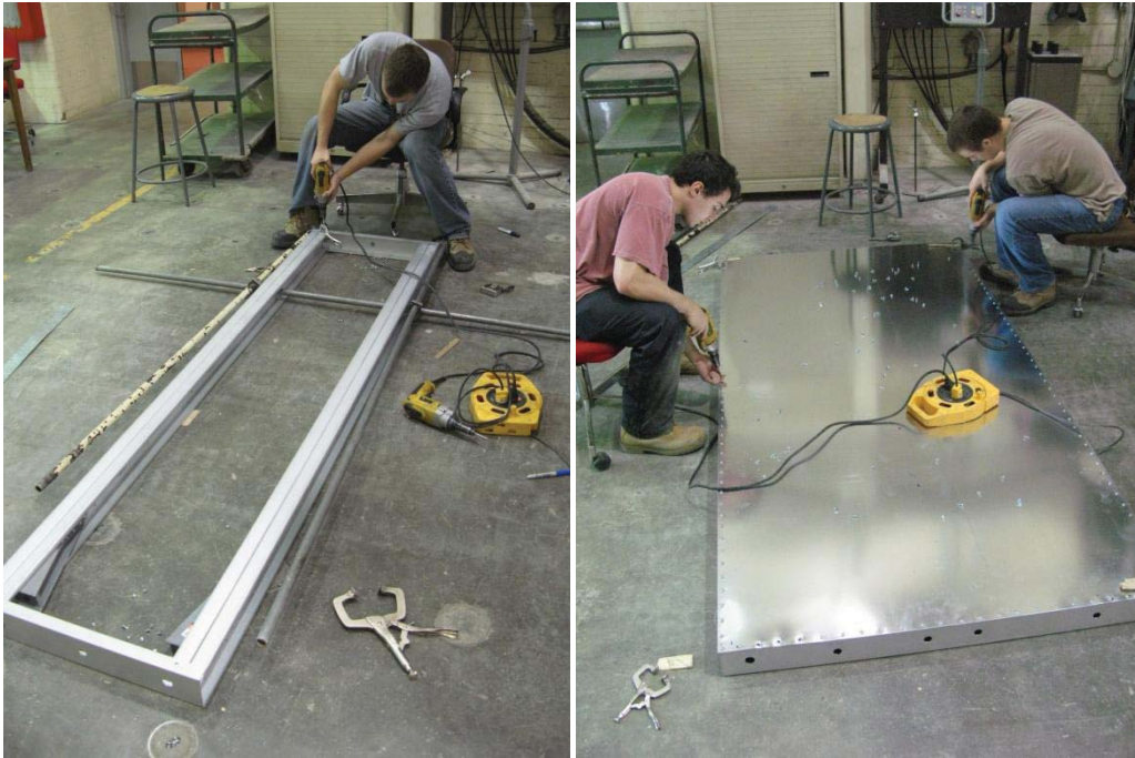
Figure 2.4 Frame and Sheathing Assembly
