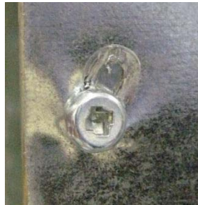
Figure 2.17 Sheathing Steel Bearing
