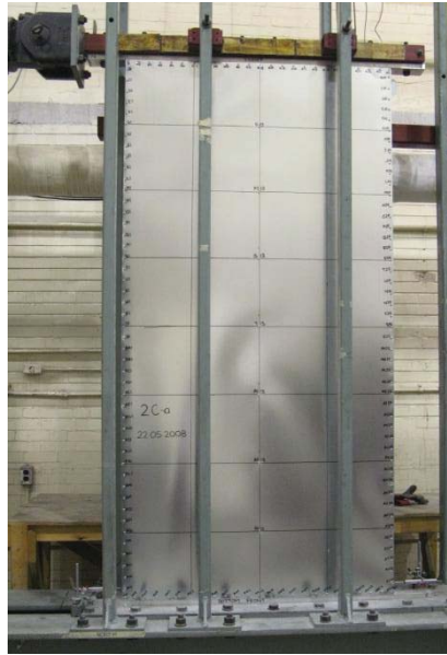
Figure 2.11 Wall Specimen before Shear Buckling and Tension Field Action
