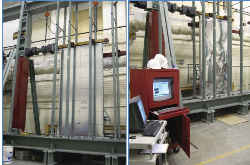
Figure 2.2 Wall Installation in Test Frame
