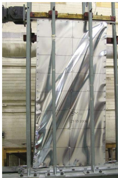
Figure 2.11 Wall Specimen before Shear Buckling and Tension Field Action
