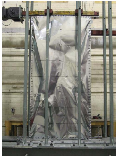
Figure 2.13 Shear Buckling and Tension Field of Sheathing in a Reversed Cyclic Test
