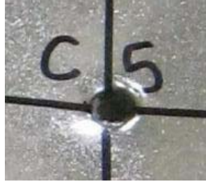
Figure 2.16 Screw Pull-Through Sheathing Failure
