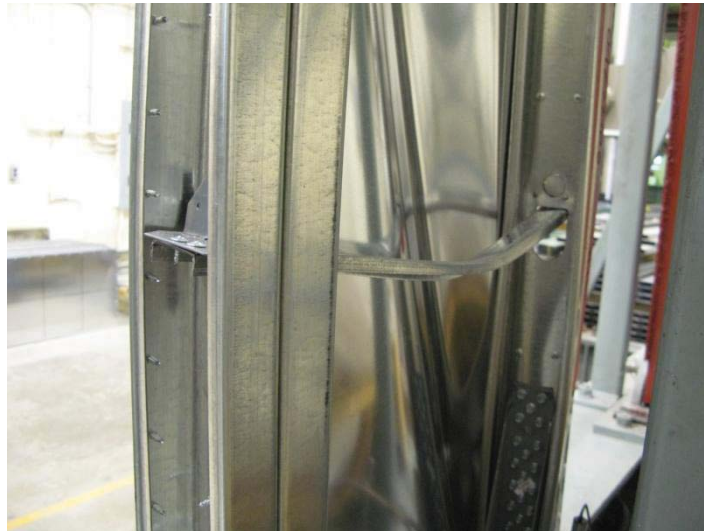
Figure 2.21 Flexural Buckling of Bridging in Test 9M-c
