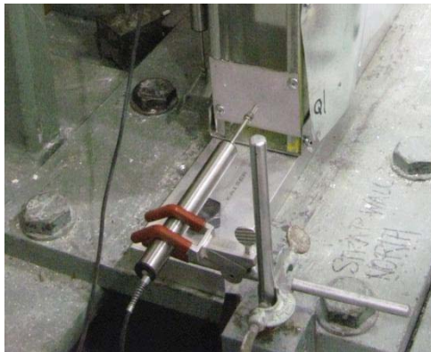
Figure 2.7 LVDT Placement on Side Plate
