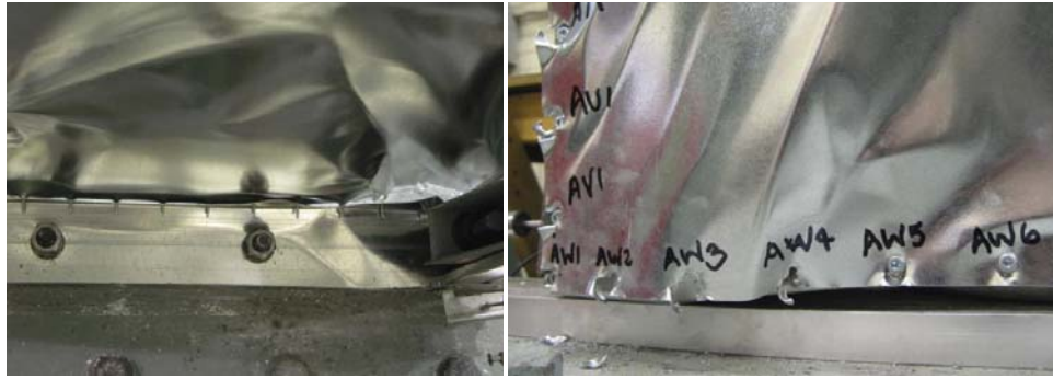
Figure 2.23 Uplift of Bottom Track
