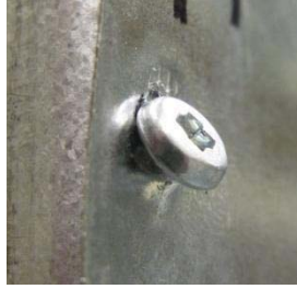
Figure 2.14 Sheathing Screw Tilting
