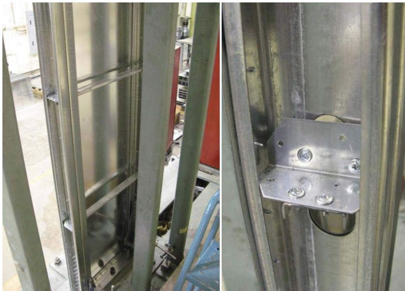
Figure 2.5 Bridging and Bridge Clip in Test 9M-c
