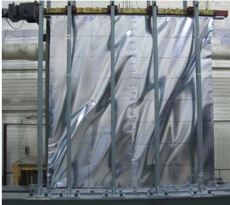
Figure 2.24 Tension Field of a Monotonic Long Wall
