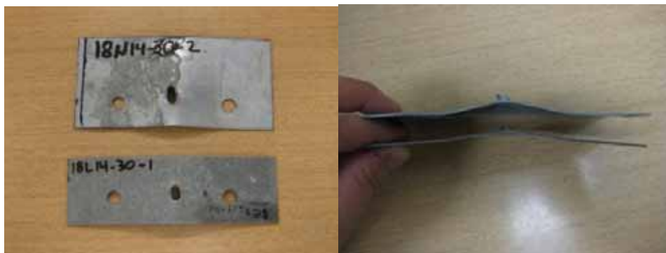
Figure 3.15 Comparison of Normal- and Low-Ductility Flat Sheets
