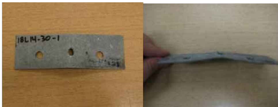
Figure 3.16 Typical Low-Ductility Flat Sheet after Testing
