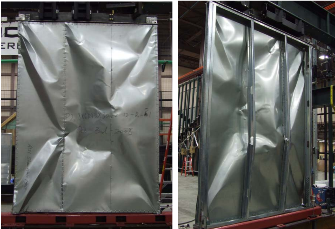
Figure 19 Failure mode of test 8x6x350-43x30-2-C1-B
