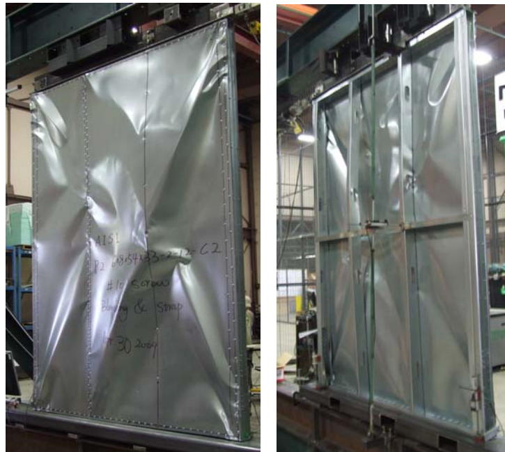
Figure 24 Failure mode of test 8x6x350-54x33-2-C2-C
