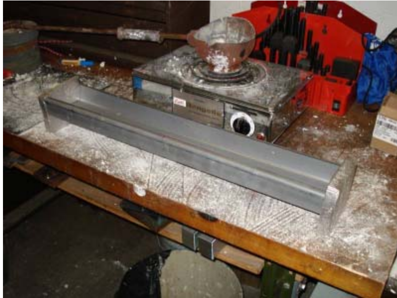
Figure 5.7 362S162-33 short column specimen with bismuth end diaphragms
