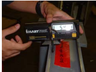
Figure 5.14 Procedure for measuring flange-lip and flange-web angles
