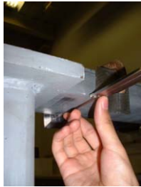
Figure 5.13 Procedure for measuring specimen cross-section dimensions
