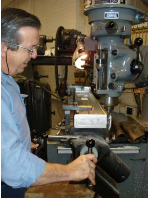
Figure 5.10 The intermediate length specimens were end-milled in a manual milling machine
