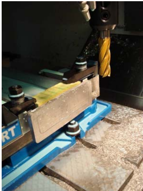
Figure 5.9 An end mill is used to prepare the column specimens
