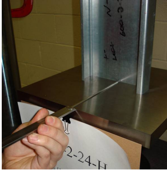
Figure 5.25 Digital calipers are used to measure the distance from the column web to platen edge
