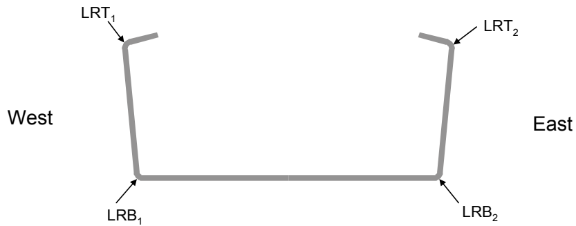
Figure 5.19 Lengths are measured at the four corners of the C-section column
