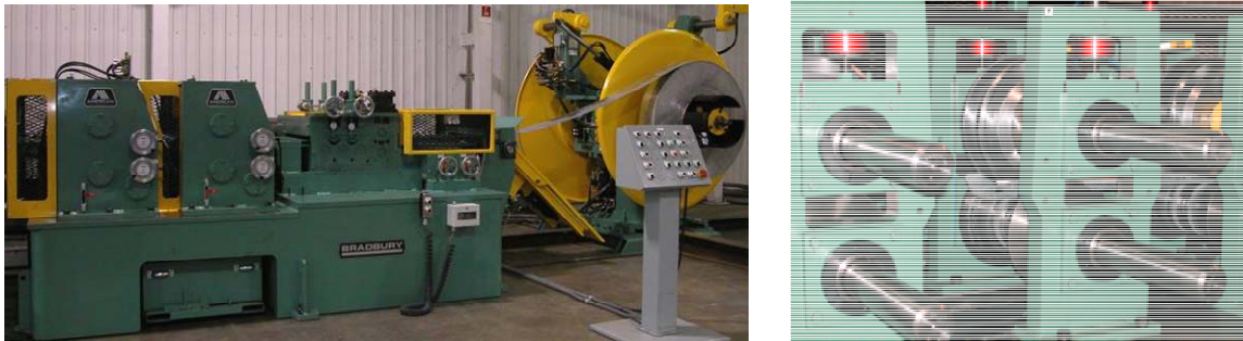
Figure 6.1 Cold-formed steel roll-forming: (left) Sheet coil enters roll-forming line, (right) steel sheet is cold-formed into C-shape cross-section (photos courtesy of Bradbury Group).
