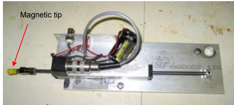
Figure 5.5 Novotechnik position transducer with ball-jointed magnetic tip
