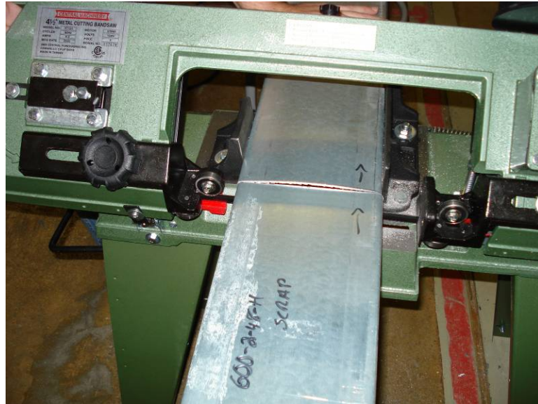
Figure 5.6 Central Machinery metal band saw used to rough cut column specimens
