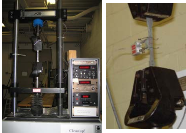
Figure 5.29 ATS machine used to test tensile coupons
