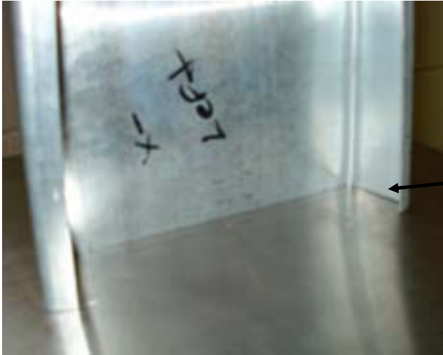
Figure 5.51 Short 600S162-33 column flange-lip corner lifts off platen during post-peak portion of test
