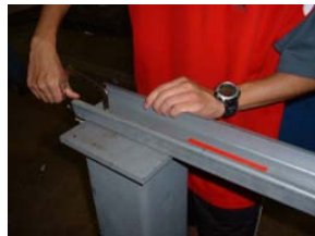
Figure 5.12 Setup procedure for measuring specimen cross section dimensions
