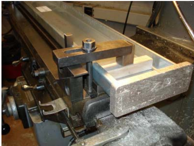
Figure 5.11 The specimens are clamped at the webs only to avoid distortion of the cross-section
