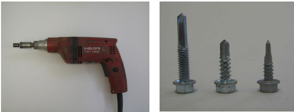
Figure 4-3: Screw Gun and Self-Drilling Screws
