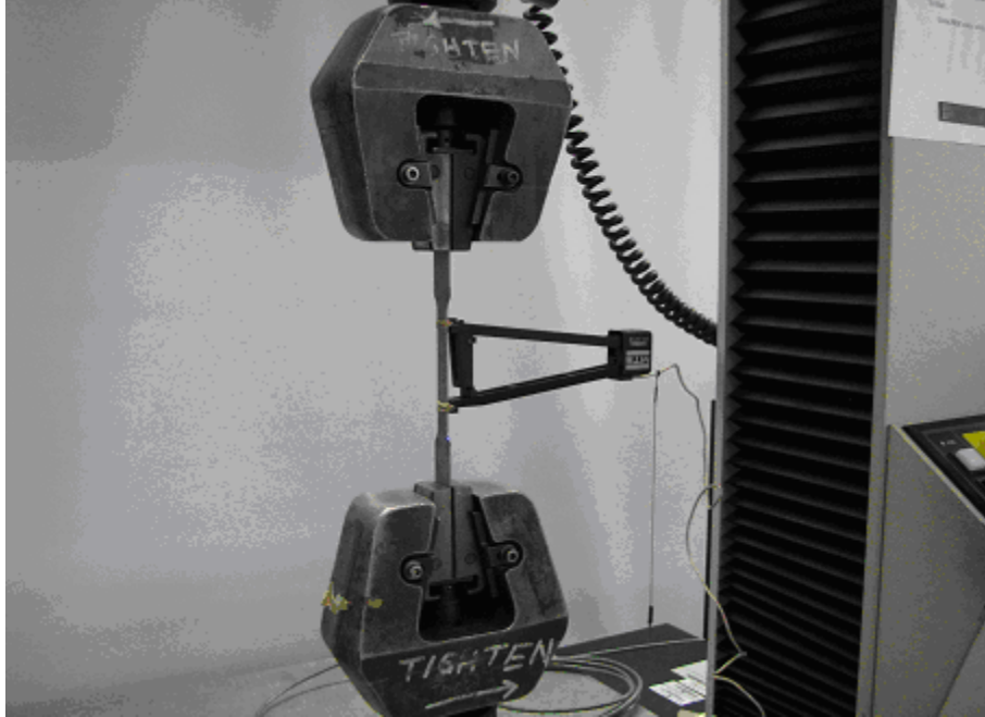
Figure 3-12: Tensile Coupon Test Setup
