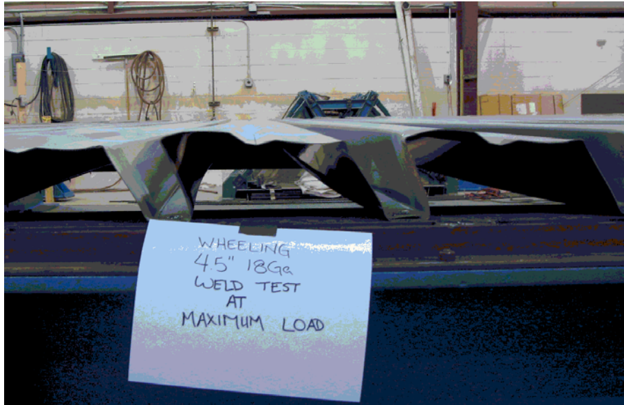
Figure 4-13: Warping distortion of N-Deck
