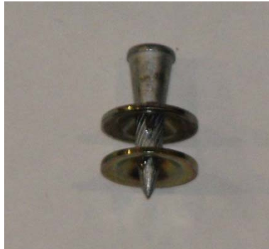
Figure 4-4: Hilti X-ENP-19 L15 Powder Actuated Fastener
