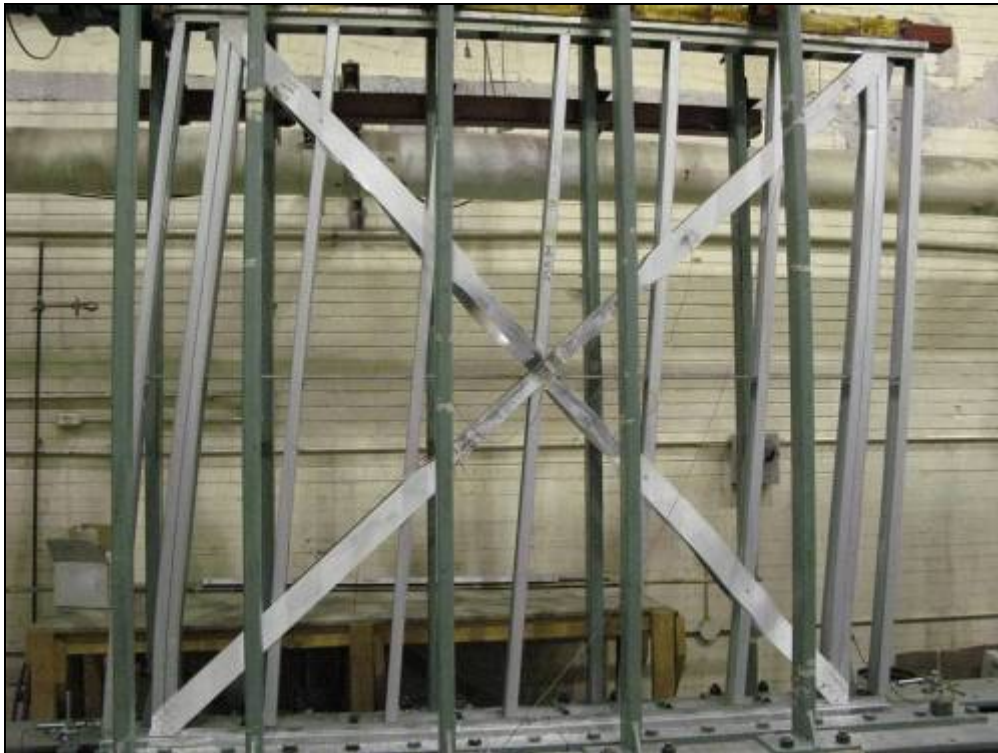
Figure 2.51 Typical wall at the end of a monotonic test (test specimen 25 A-M 1)
