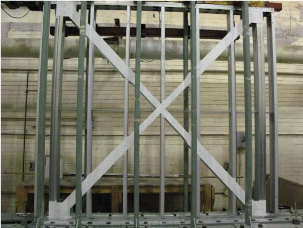
Figure 2.26 Strap braced wall specimen 27 A-M in test frame
