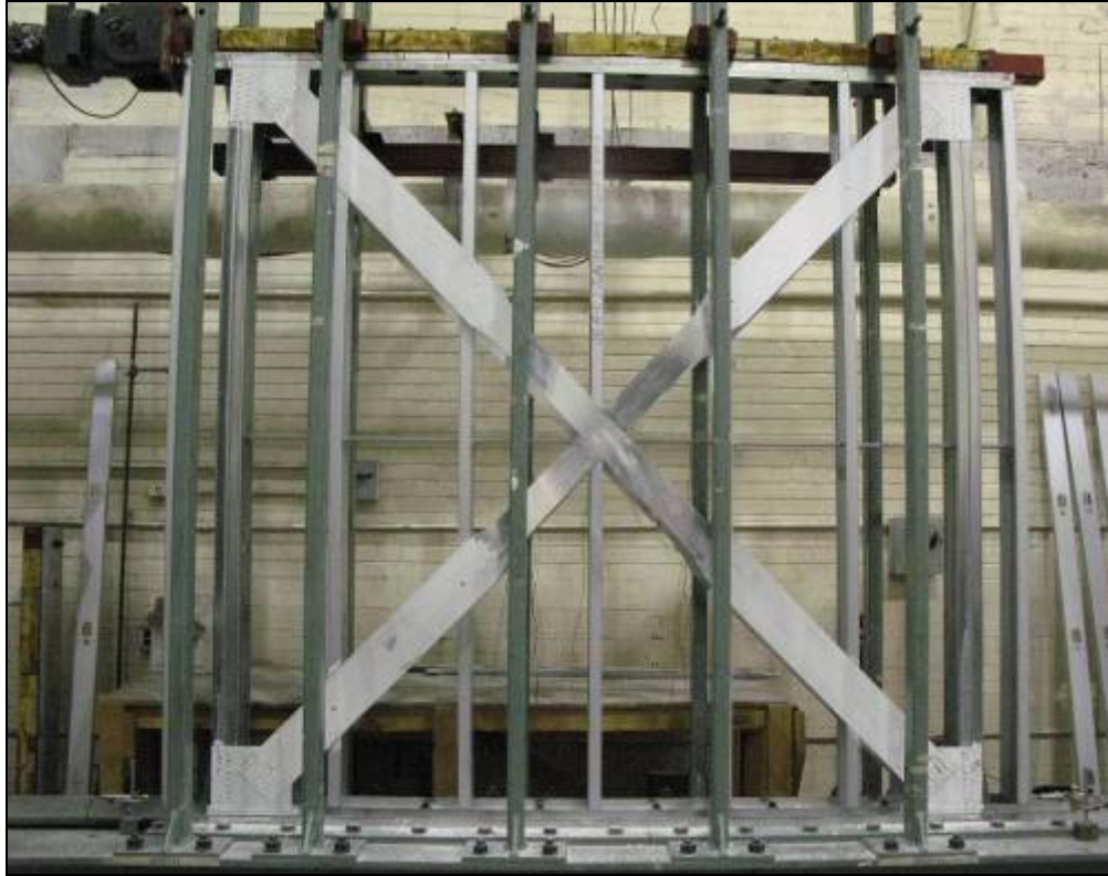
Figure 2.50 Test Specimen photographs showing elongated fuse section
