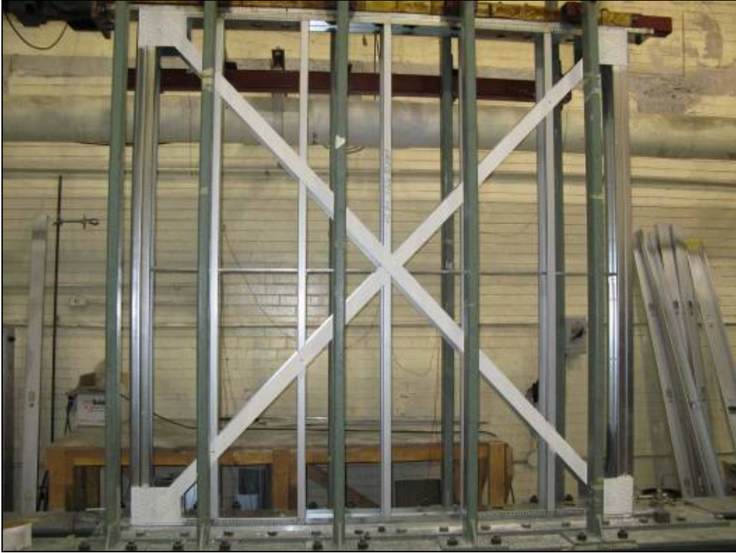
Figure 2.28 Strap braced wall specimen 40 A-C in test frame
