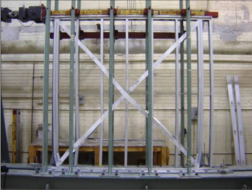
Figure 2.58 Bending of chord studs of specimen 36A-C
