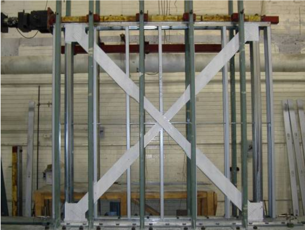
Figure 2.36 Strap braced wall specimen 30 A-C in test frame
