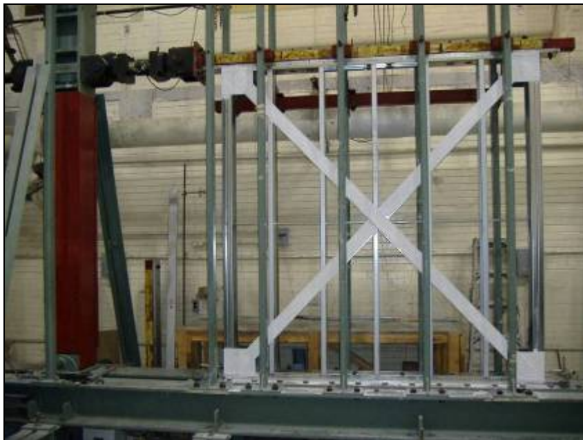
Figure 2.1 Strap braced wall specimen 46A-C in test frame
