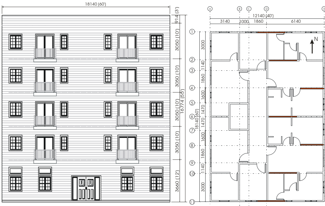
Figure 3.1 West elevation and plan view of the representative building (Cobeen et al., 2007), mm (ft)
