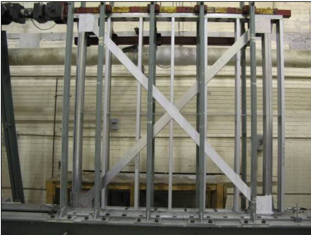
Figure 2.39 Strap braced wall specimen 37 A-M in test frame
