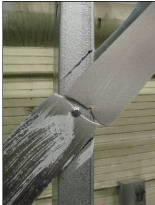
Figure 2.55 Lüder's band lines (left) and net cross-section failure of a brace (right) of specimen 31A-M 2 at 4.5% drift
