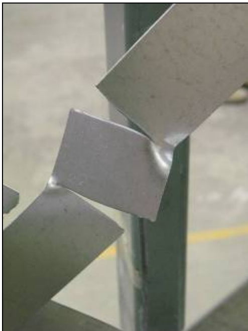
Figure 2.53 Net section fracture of braces of specimen 27A-M 1 at 8.6% drift
