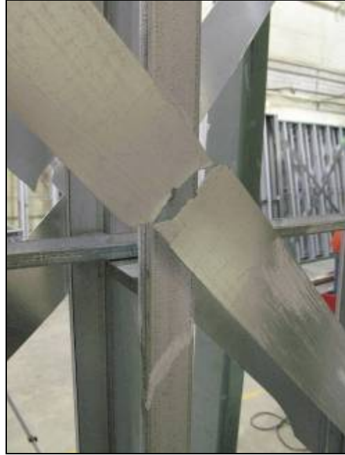
Figure 2.54 Net section fracture of braces of specimen 27A-M 2 at 3.6% drift
