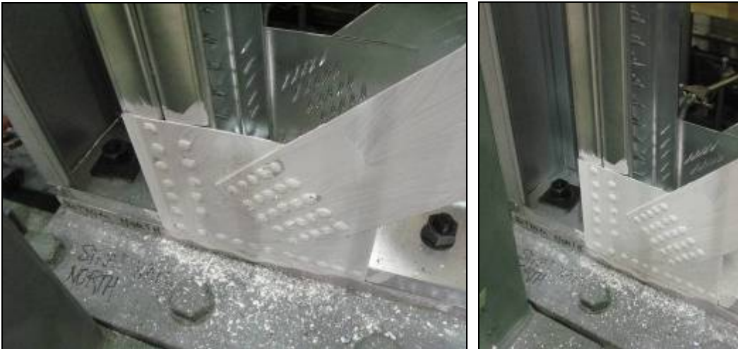
Figure 2.27 Holddown detail of specimen 27 A-M
