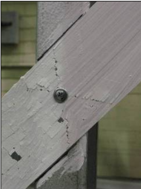
Figure 2.55 Lüder's band lines (left) and net cross-section failure of a brace (right) of specimen 31A-M 2 at 4.5% drift
