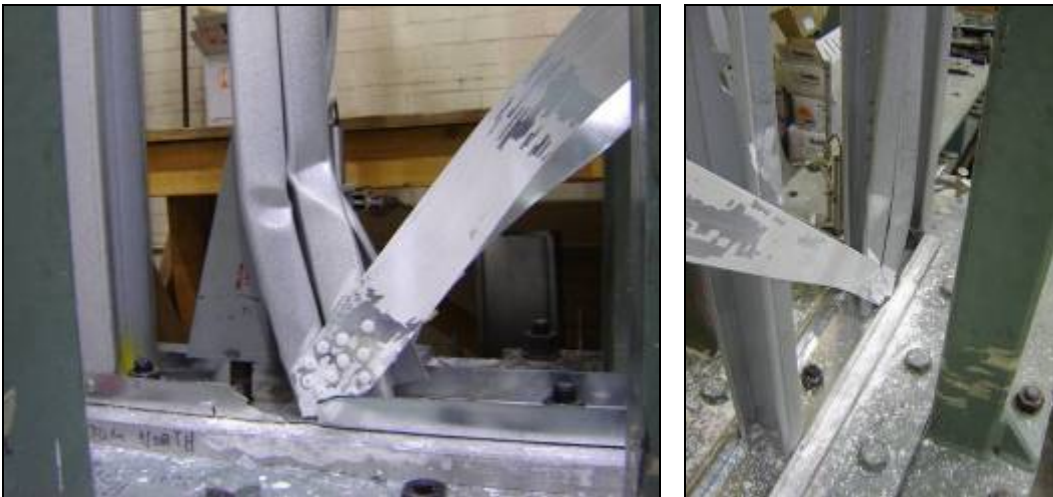
Figure 2.59 Block shear failure of flanges of the bottom track and bending of chord studs of specimen 36A-C
