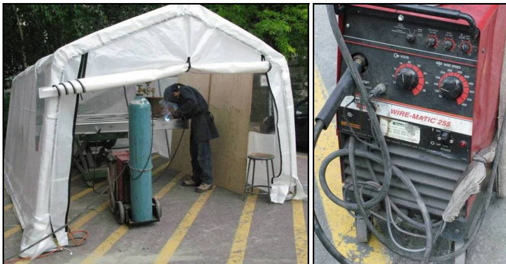
Figure 2.5: Welding setup and Lincoln Electric GMAW welder
