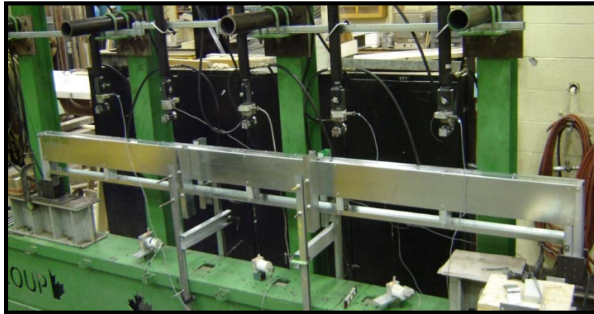
Figure 1.8 Gravity Load Case - Long Span Test Setup
