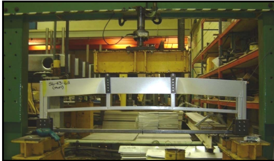
Figure 3.1 Uplift Load Case - Buckling Failure of Web Section (6' Assemblies)
