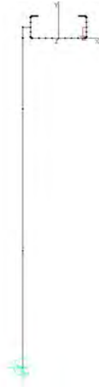
Figure 1 Mastan model with fastener beam element
