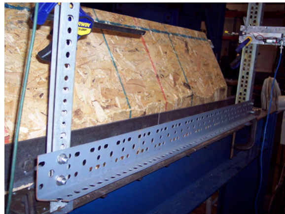
Figure 53 Sheathing Fracture Failure
