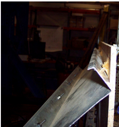
Figure 52 Fastener Pullout Failure
