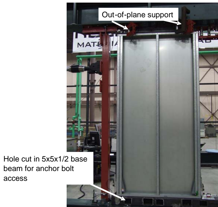
Figure 2 Back view of the test setup
