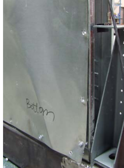
(b) test 4×8×43×33-6/12-C1 with No. 8 screws
