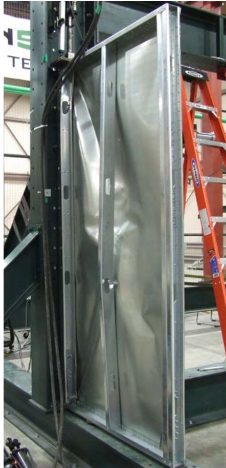
Figure 25 Set up for axial compression test
