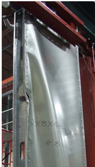
Figure 15 Buckling of double studs for 2-ft. x 8-ft. walls with 2 1/2" screw spacing
