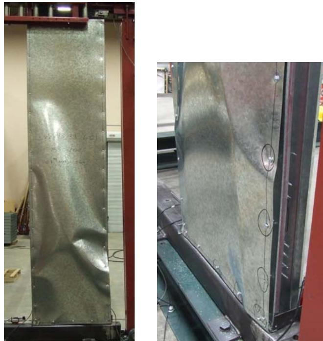
Figure 21 Failure mode for test 2x8x43x33-6-C1
