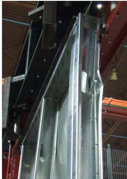
Figure 24 Observed stud failure in test A-5
