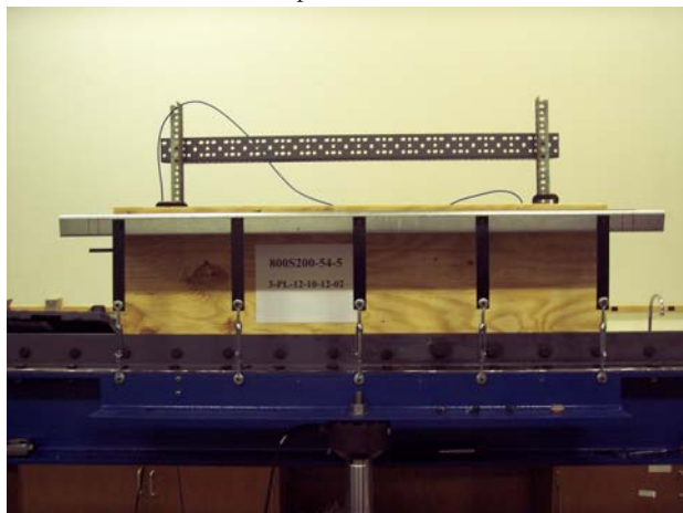
(c) testing rig with L=12 in. plywood specimen in place, actuator attached to angle which is attached to loading straps with turnbuckles and bolted to joist flange
