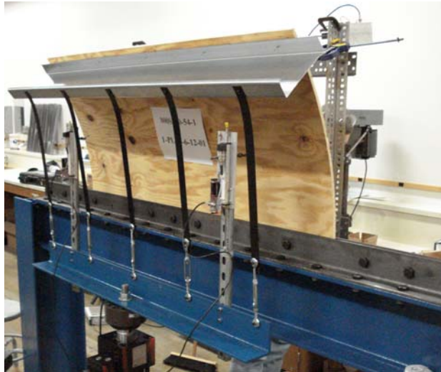
(a) typical response of plywood sheathed joist shown for an 800S200-54 joist with plywood, L = 24 in., and #6 fasteners @ 12 in. (1-PL-24-6-12-01_A, 1-800S200_54_1A)
