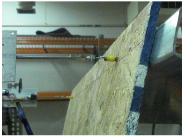
(f) final transducer to sheathing connection using short wire and magnet connection to a fastener
