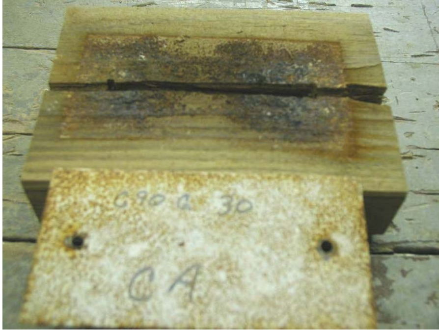
Photo 21 – Specimen in CA Treated Wood After 30-Days
