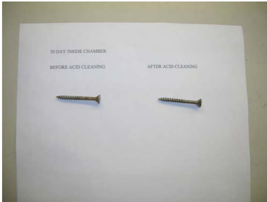
Photo 35 – Fastener Specimen After Testing – 30-Day
