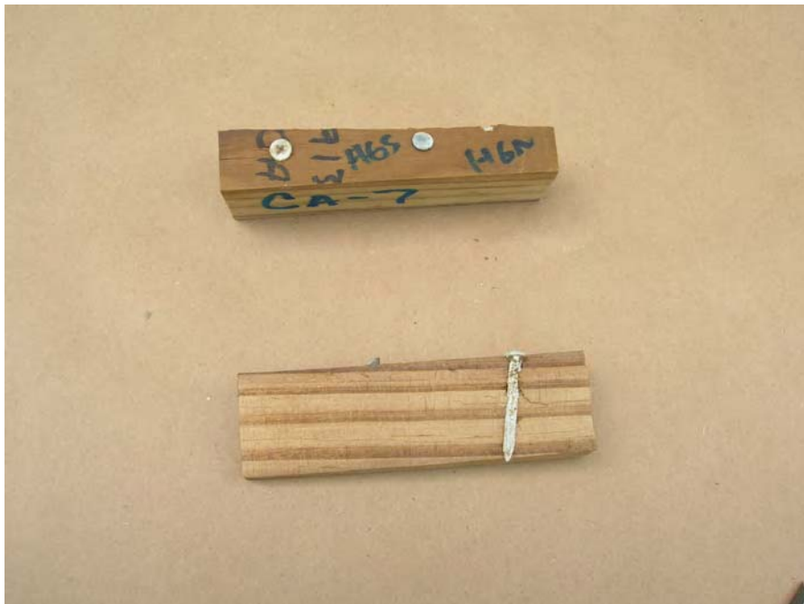
Photo 30 –Fastener Specimen After Testing – 15-Day
