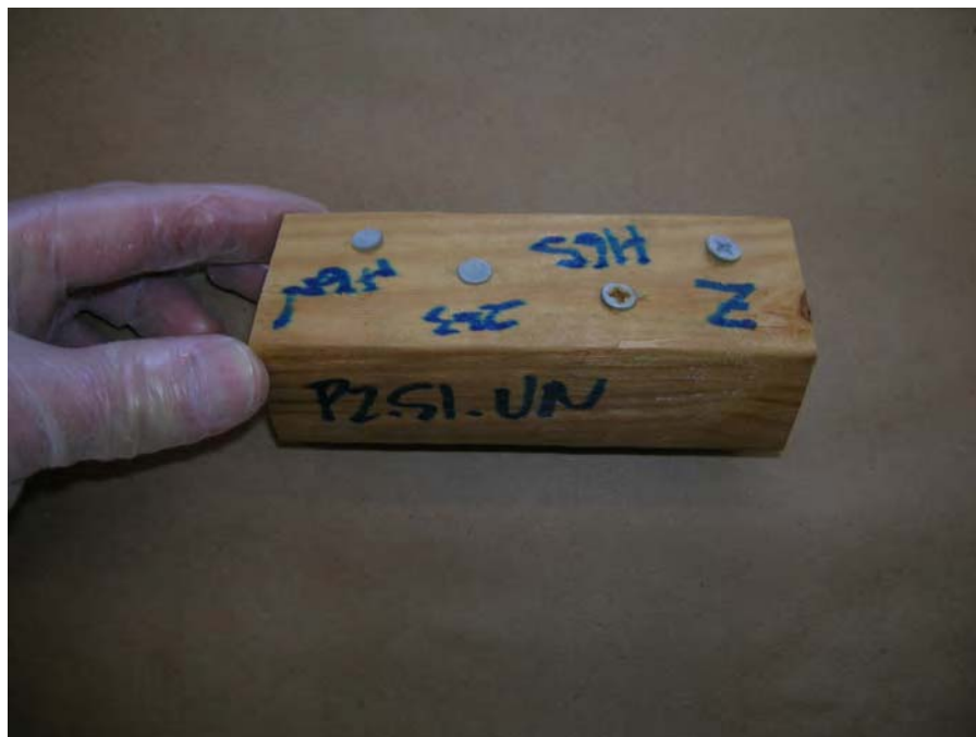
Photo 38 –Fastener Specimen After Testing – 30-Day
