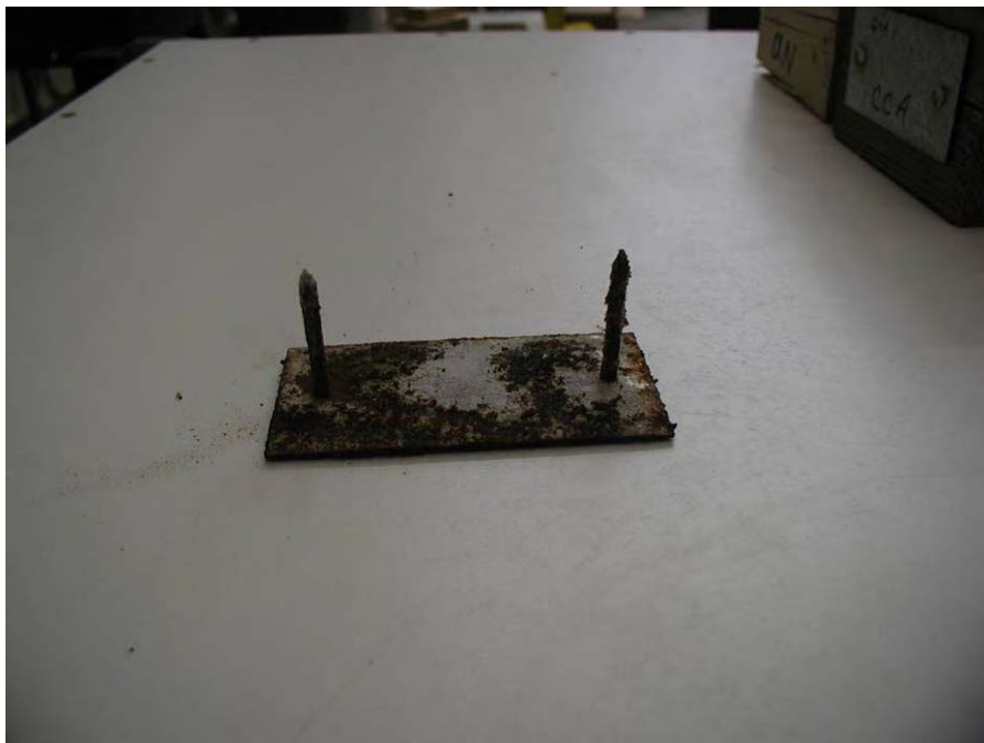
Photo 26 – Contact Side of CA Treated Sample (30-Days)
