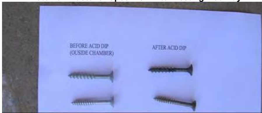
Photo 46 –Fastener Specimen After Testing – 90-Day
