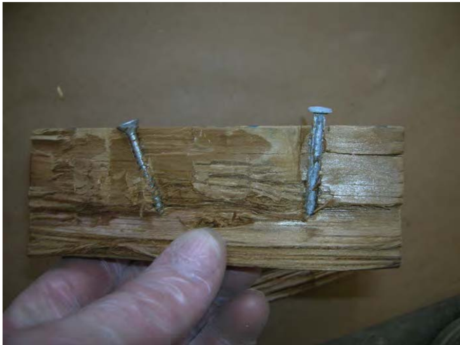
Photo 36 –Fastener Specimen After Testing – 30-Day
