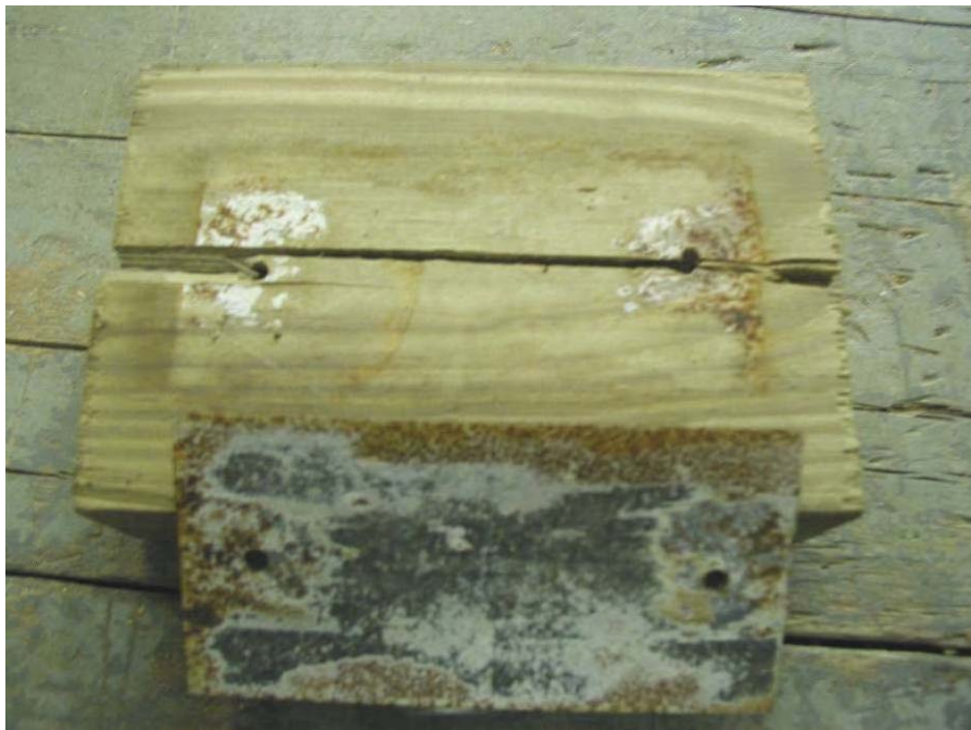
Photo 22 – Specimen in ACQ Treated Wood After 30-Days
