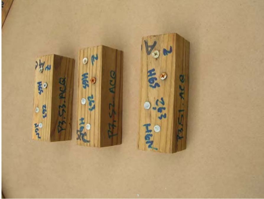
Photo 29 – Fastener Specimen After Testing – 15-Day
