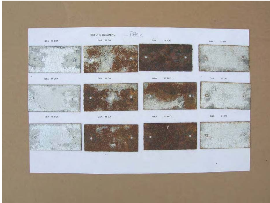
Photo 27 – Back of Specimens Before Cleaning (30-Days)
