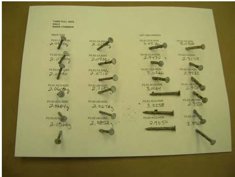
Photo 33 – Fastener Specimen After Testing – 15-Day
