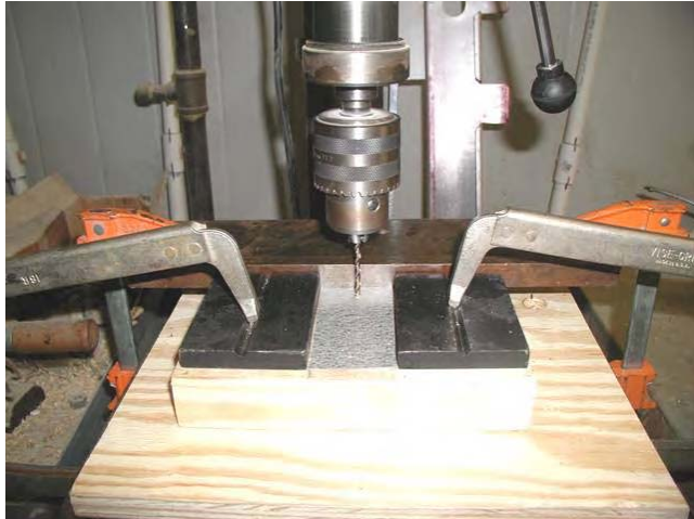
Photo 5 – Pre-Drilling Holes in Steel Coupons
