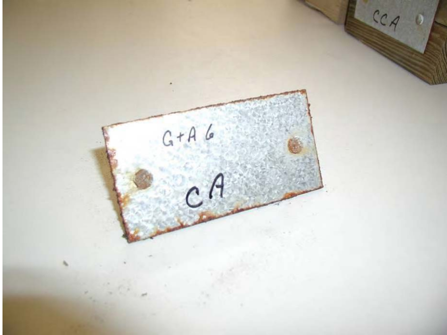
Photo 25 – Exposed Side of CA Treated Sample (30-Days)
