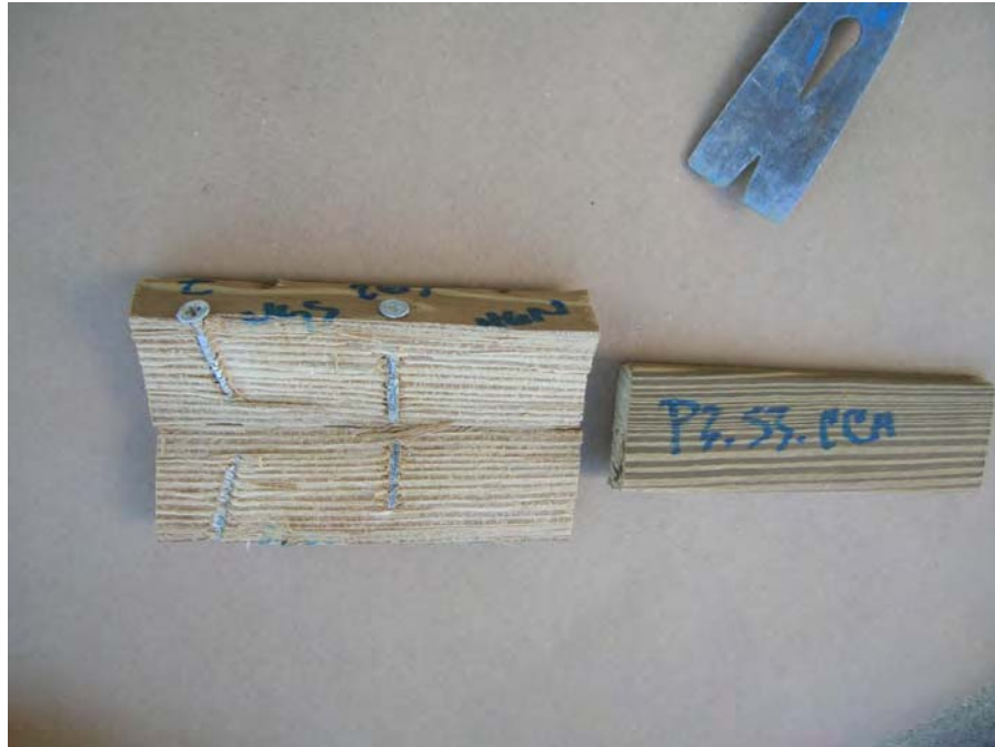
Photo 31 – Fastener Specimen After Testing – 15-Day
