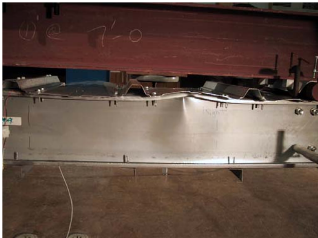
(b) t = 0.043 in. nominal (test 8C043-5E6W)
