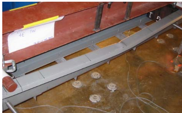
(b) Distortional buckling test
