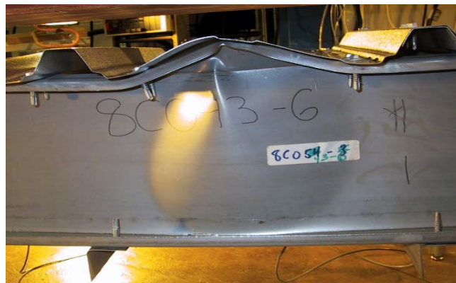
(a) Local buckling test
