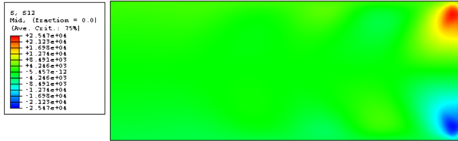
Figure 6.43 Stress \tau_{xy} distribution (at peak load, on mid-surface) of a ss-ss stiffened element under a stress gradient r = 0
