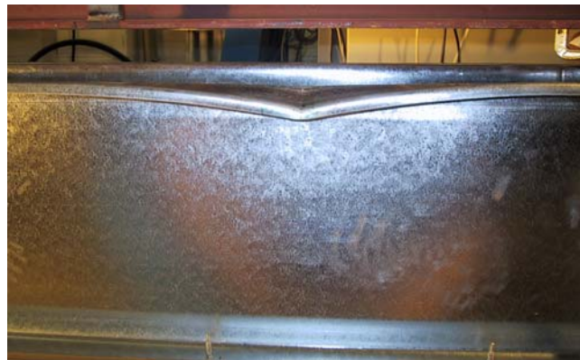
(b) Distortional buckling test
