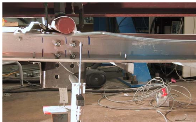
(b) Distortional buckling test
