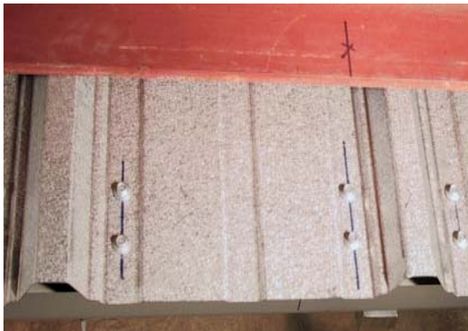
Figure 2.19 Fastener configuration C for test 8.5Z073-4E3W
