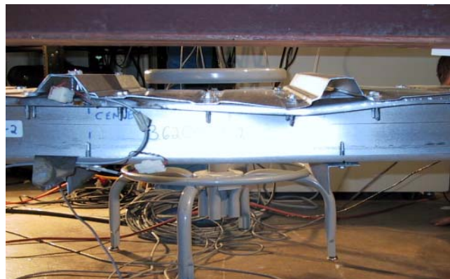
(a) Local buckling test
