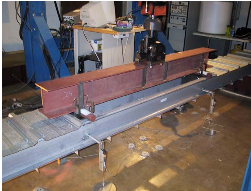
Figure 3.3 Panel setup for distortional buckling tests
