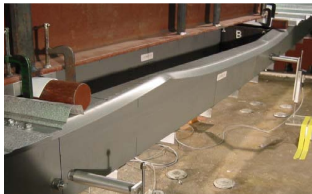
(b) Distortional buckling test
