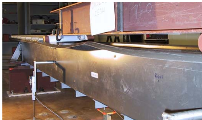
(b) Distortional buckling test of D11.5Z092-3E4W
