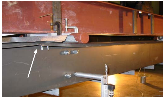
(a) Local failure begins
