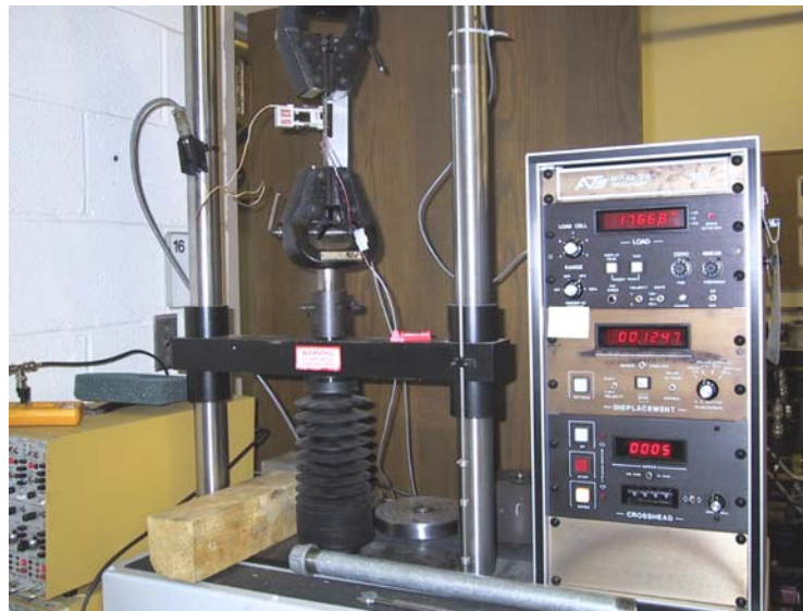
Figure 4.2 Overall view of tension test setup
