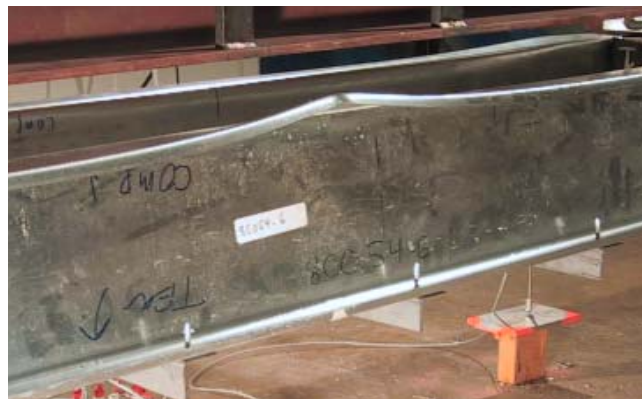
(b) Distortional buckling test
