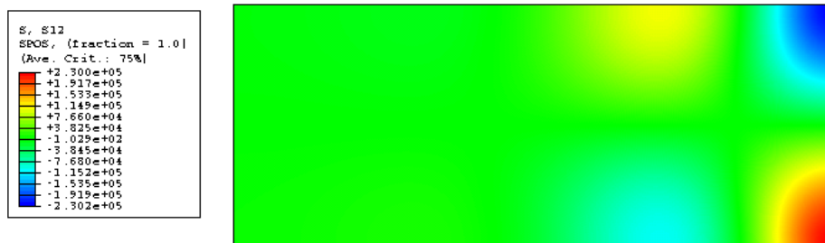
Figure 6.11 Stress \tau_{xy} distribution on top surface of a ss-ss stiffened element under a stress gradient r = 0 by elastic FE solution
