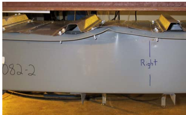
(a) Local buckling test
