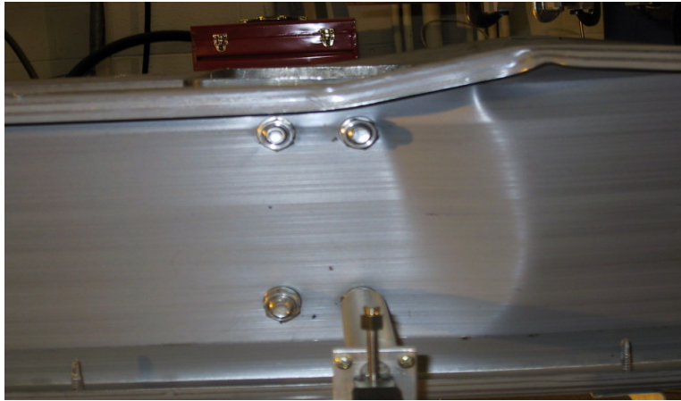
Figure 3.37 Failure of test D8C033-1E2W
