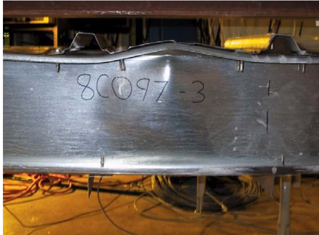
(a) t = 0.097 in. nominal (test 8C097-2E3W)
