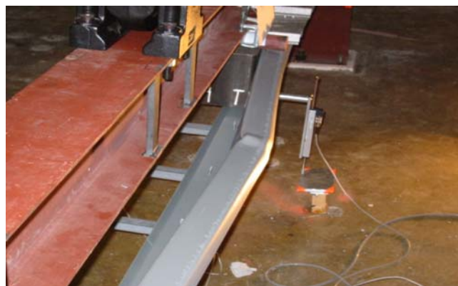
(b) Distortional buckling test
