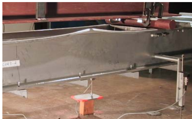
(b) Distortional buckling test
