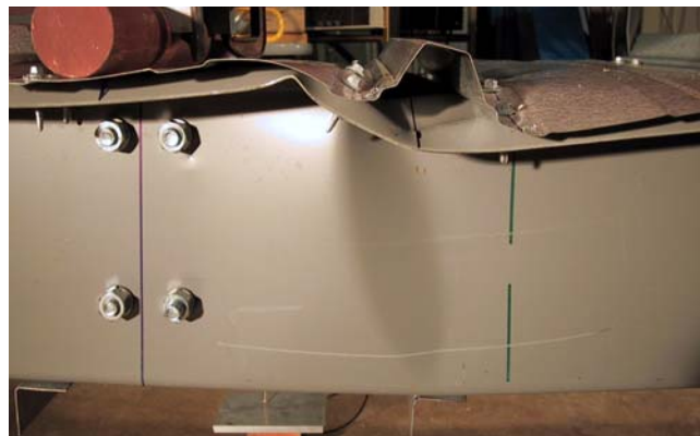
(a) Local buckling test
