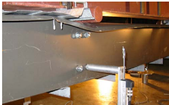
(b) Distortional buckling test
