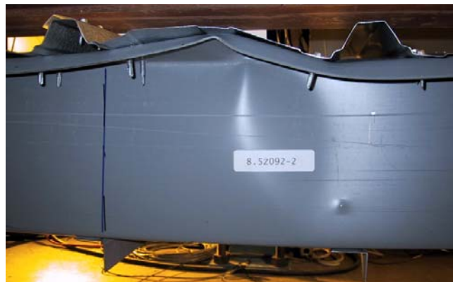
(a) Local buckling test
