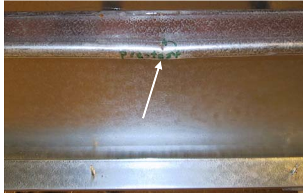
(a) Pre-test damage
