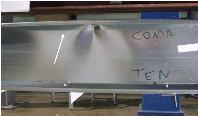
Figure 3.38 Failure of test D10C056-3E4W
