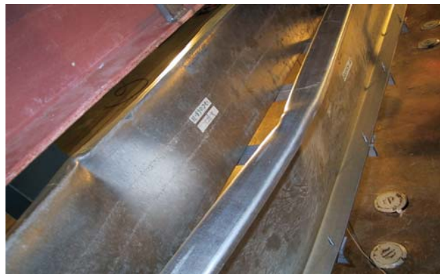
(b) Distortional buckling test
