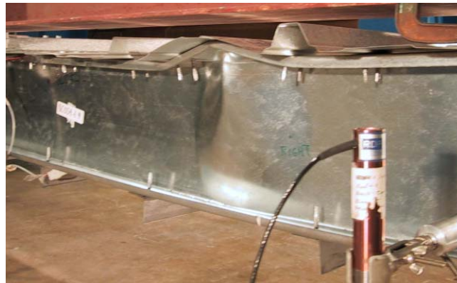
(a) Local buckling test
