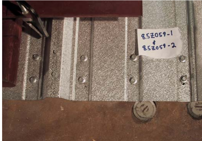
Figure 2.20 Fastener configuration D for test 8.5Z059-2E1W
