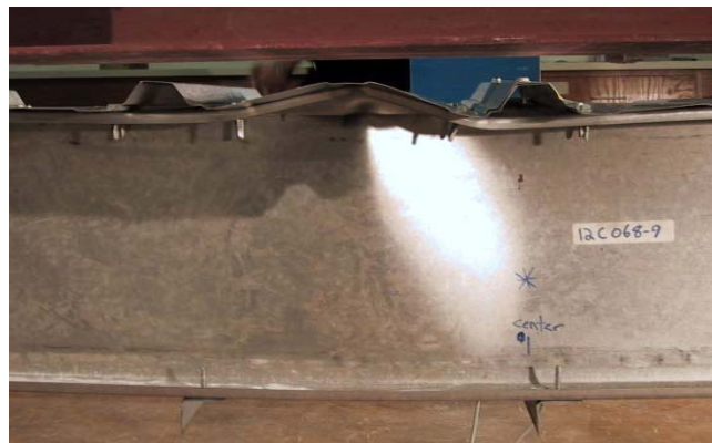
(a) Local buckling test
