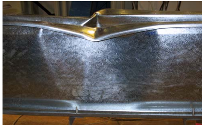
(a) Local buckling test
