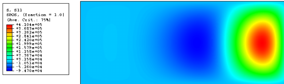
Figure 6.10 Stress \sigma_x distribution on top surface of a ss-ss stiffened element under a stress gradient r = 0 by elastic FE solution
