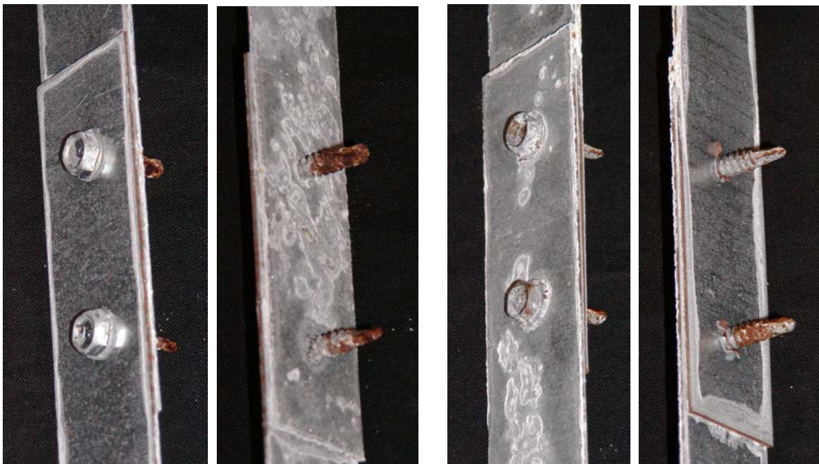
Figure 6.23: Test connections after 1537 cycles – Threads up (left) and down (right)
