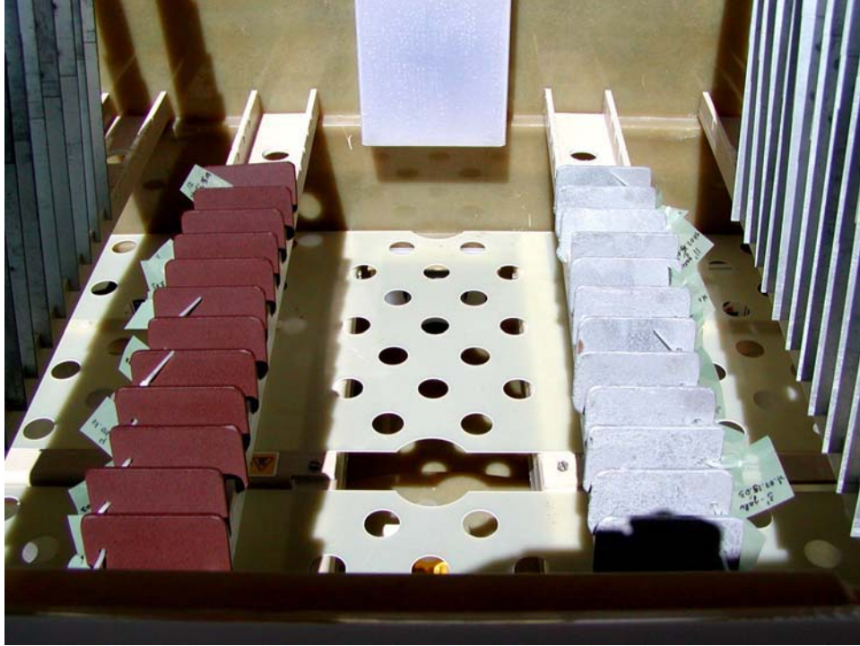
Figure 5.10: Steel and zinc coupons after 5 days in the corrosion chamber (160 cycles)
