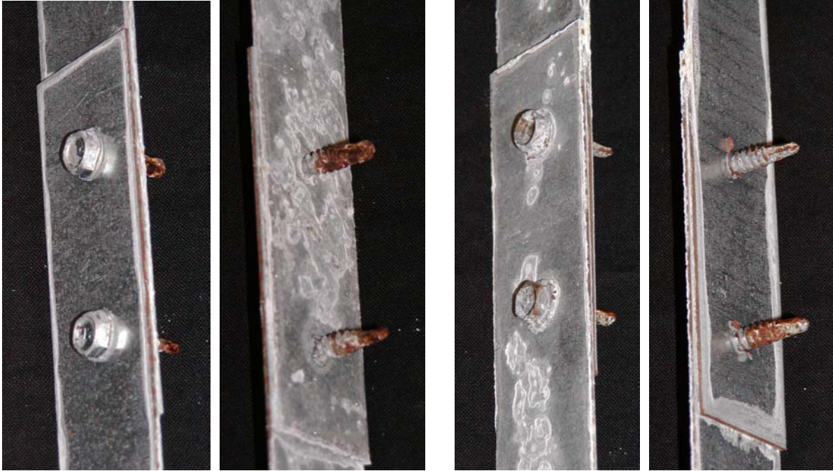
Figure 6.20: Test connections after 1309 cycles – Threads up (left) and down (right)
