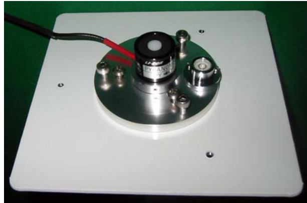
Figure 2.20: LI200S solar radiation sensor mounted on leveling plate
