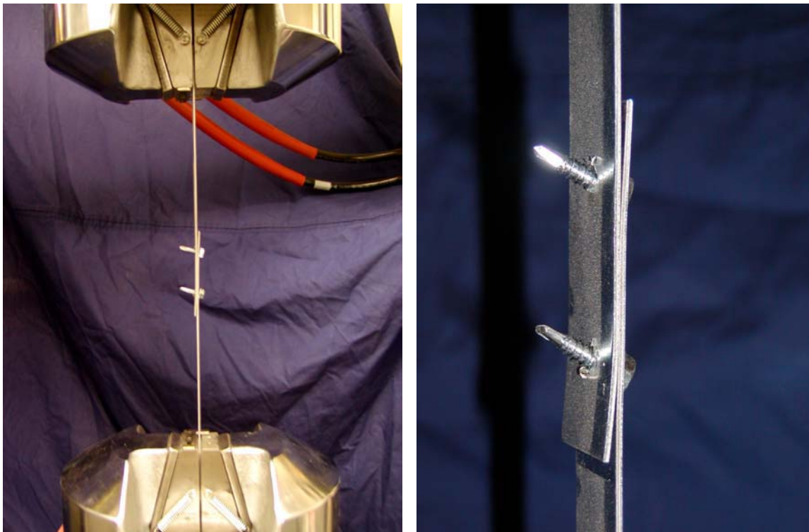
Figure 6.1: Control specimen in test frame
