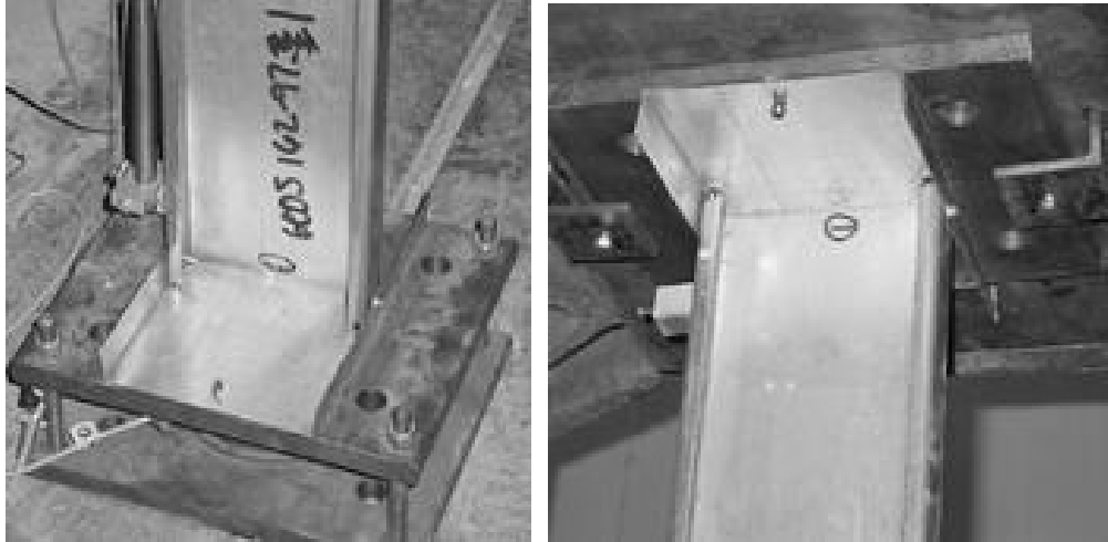
Figure 3.5 Connection of Cee-Stud and Track (a) at Top, (b) at Bottom
