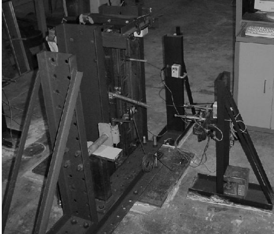
Figure 3.13 Overall View of the Out-of-Plane Bridging Tests
