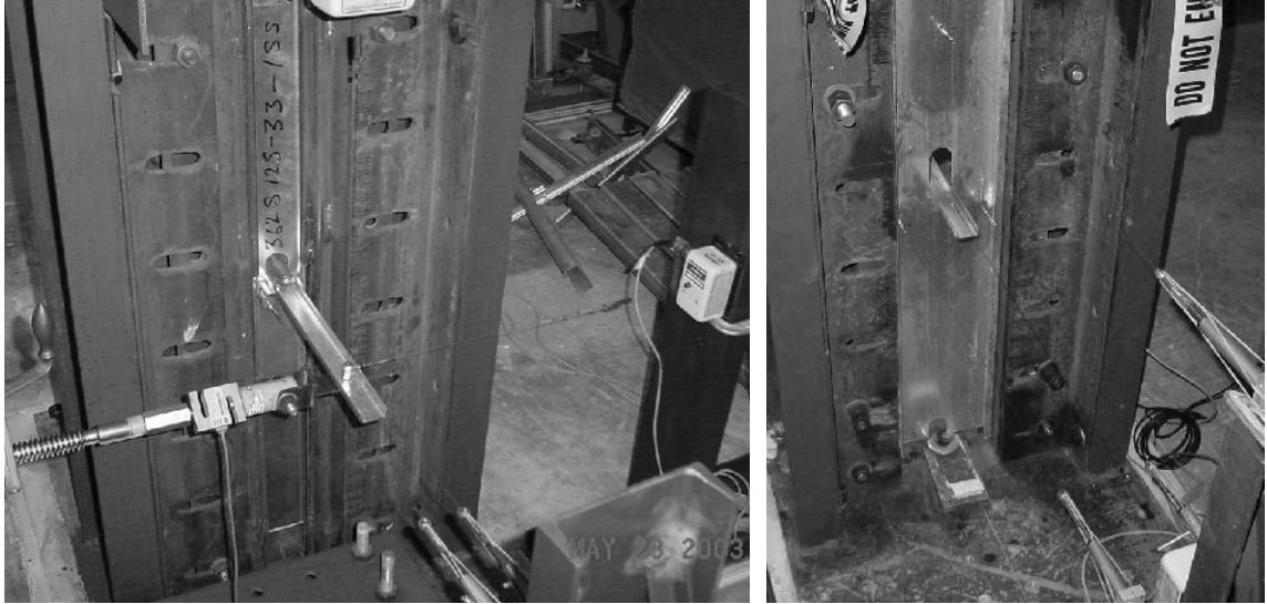
Figure 3.15 Out-of-Plane Loading Test Instrumentation on the (a) Front (b) Back
