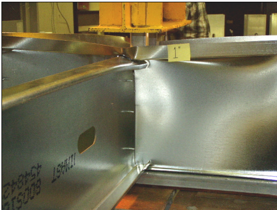
Figure 5.8: Photograph of the Deformation at 1" Deflection (Offset Loading)
