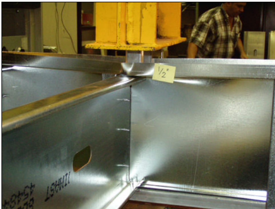
Figure 5.6: Photograph of the Deformation at \frac{1}{2} Deflection (Offset Loading)
