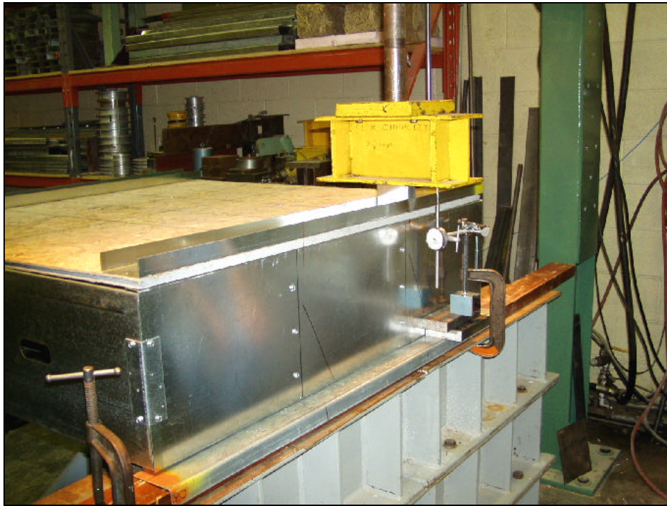
Figure 4.3: Photograph of the Test Set-Up for an End Loading
