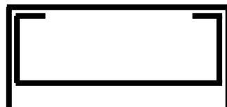
Figure 2 – Mitek's Load Bearing Top Track Configuration
