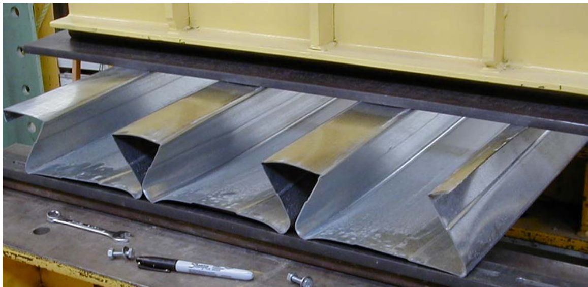
Figure 5.4-1: Failure of Re-entrant Deck Section
