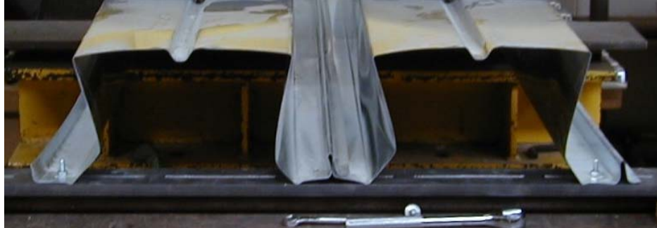
Figure 1.3-1: Typical Web Crippling Failure for Multi-Web Deck Sections
