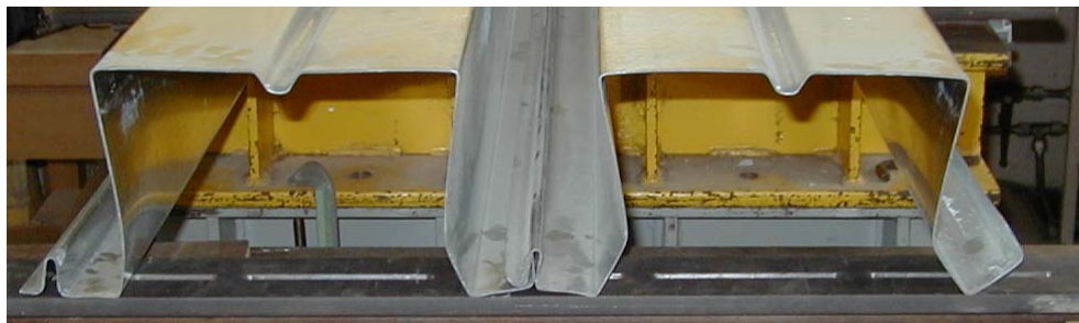
Figure 5.3-2: Photograph Showing Larger Deformation in Outside Flanges and Webs
