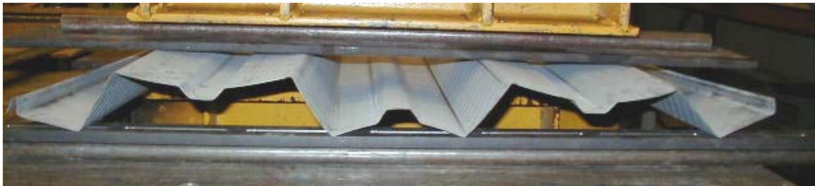
Figure 5.2-2: Spreading of a 4 Web Deck Section
