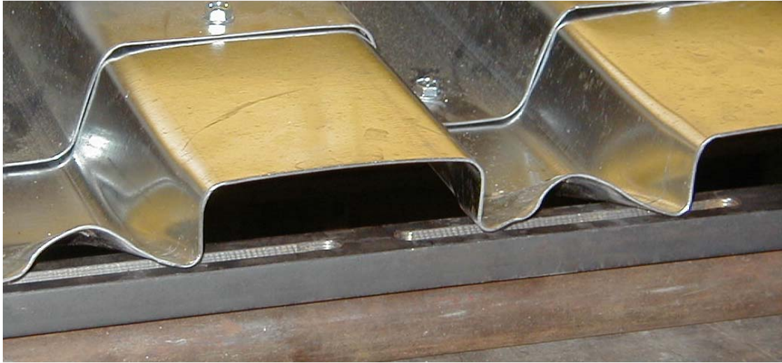
Figure 3.3-1: Specimen Reinforced to Achieve EOF Loading
