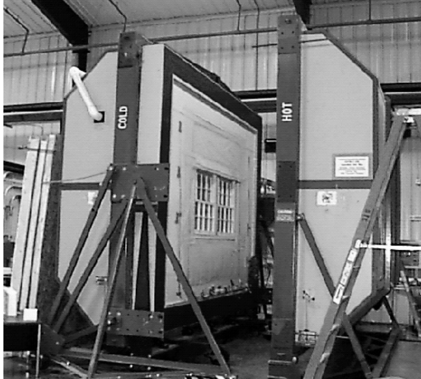
Figure 6 - Rotatable Guarded Hot Box
