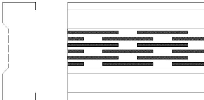
Figure 5 – Web Perforated Steel Stud Tested by Kesti
