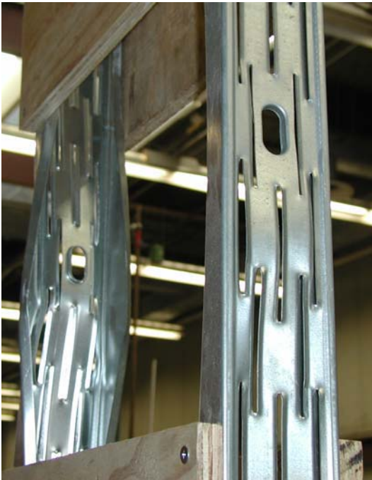
Slit-Web Stud Axial Test Setup and Failure Mode
