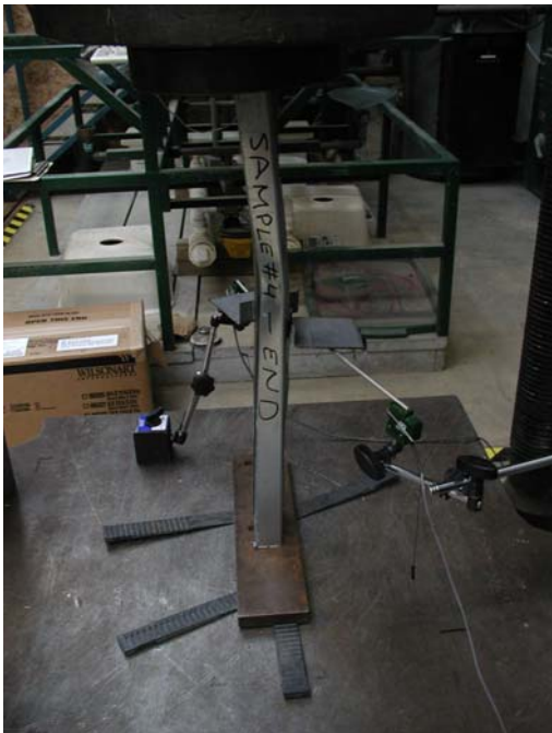
Slit-Web Stud Stub-Column Test Setup and Failure Mode
