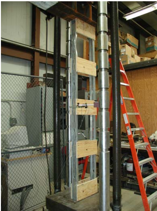
Slit-Web Stud Failure Mode in Axial Tests
