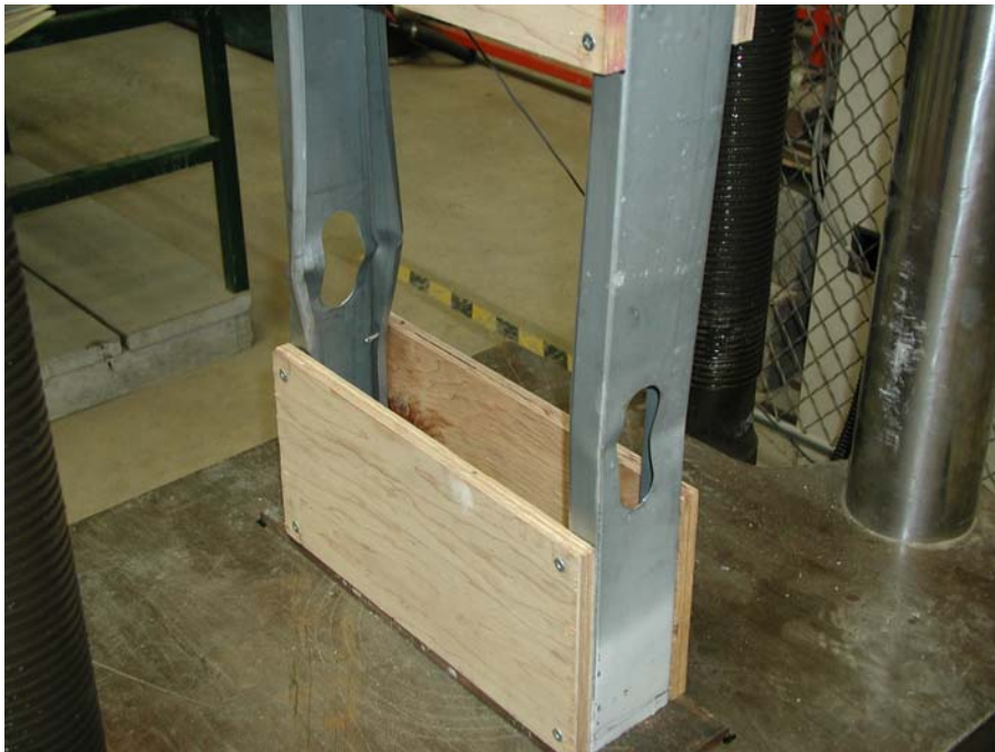
Solid Web Stud Failure Mode in Axial Tests
