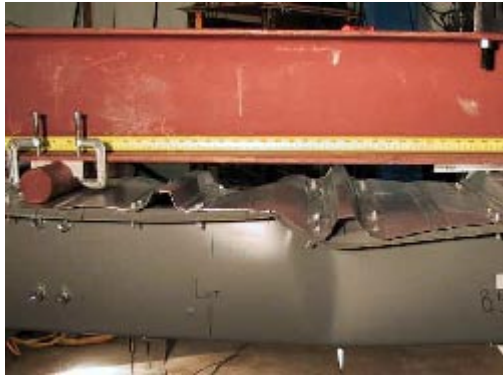
(a) Collapse of 8.5 in. Zee, t = 0.073 in. (nominal)
