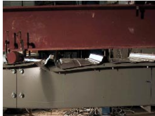
(b) Collapse of 8.5 in. Zee, t=0.059 in.(nominal)
