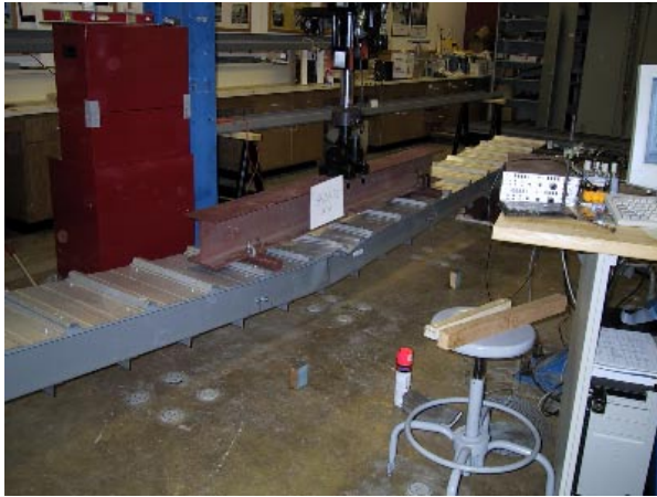
Figure 7 Overall view of failed specimen (test 8.5Z073-1E2W shown)
