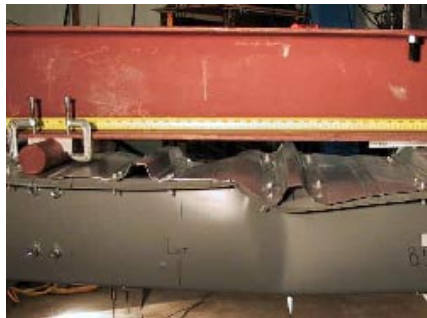
(a) Collapse of 8.5 in. Z, t=0.073 in. (nominal)
