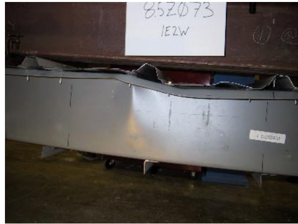
Figure 8 Close-up view of failed purlin (test 8.5Z073-1E2W shown)
