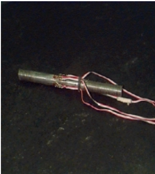
Figure 2.6 Instrumented Rods Used as Load Cells
