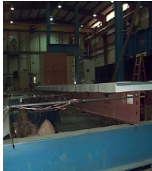
Figure 2.6 Instrumented Rods Used as Load Cells
