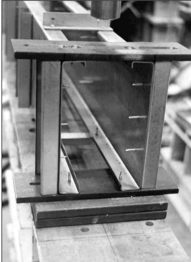
Figure 4.6.1: Fastening Joist Flanges to the Bearing Plate
