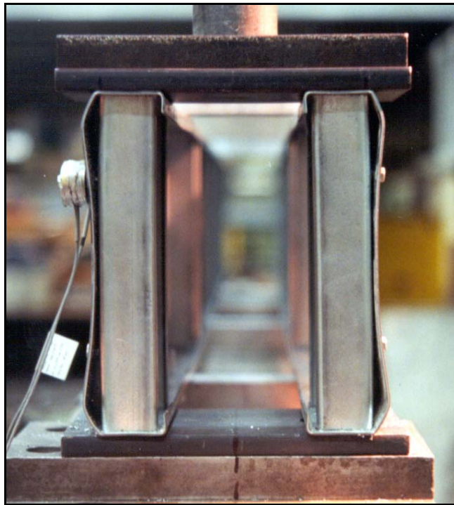
Figure 8.1.2: Photograph of the Web Crippling of a Pair of C-Sections with Bearing Stiffeners
