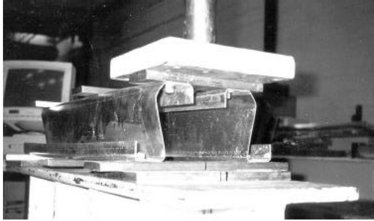
Figure 3.4 End Two Flange Loading, ETF, of Z-Sections
