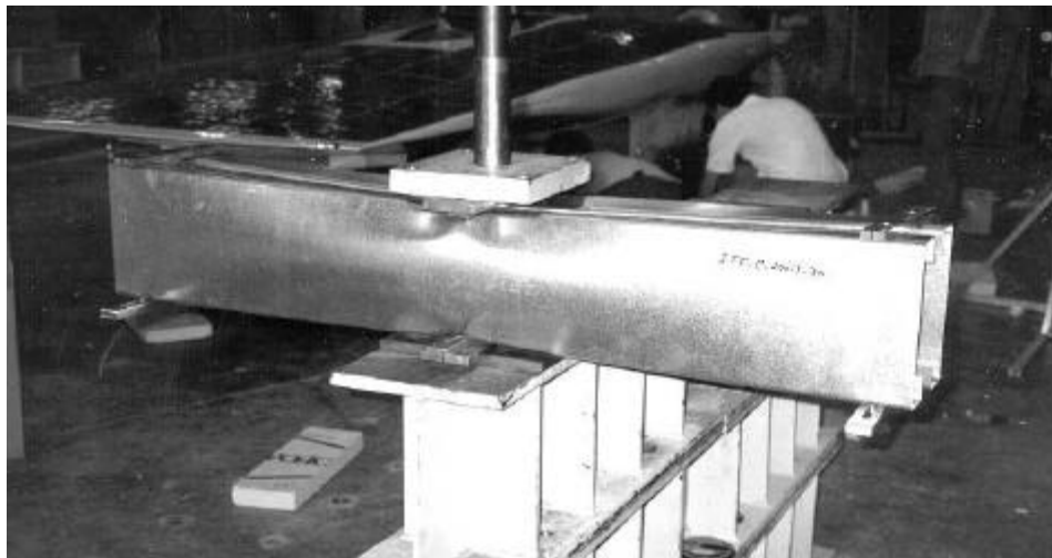
Figure 3.11 Interior Two Flange Loading, ITF, of C-Sections
