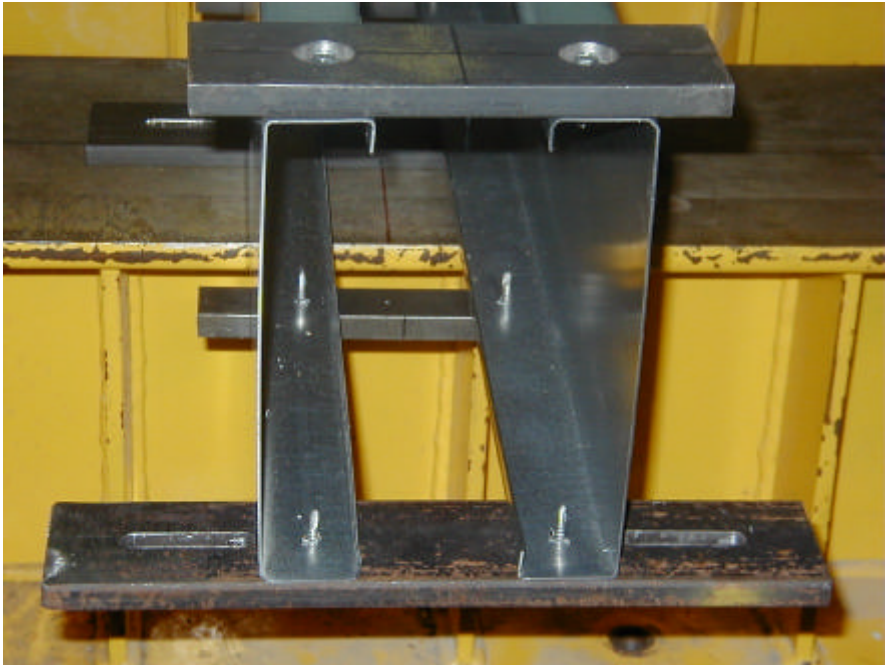
Figure 1 Screw-fastened Specimen in Test Frame
