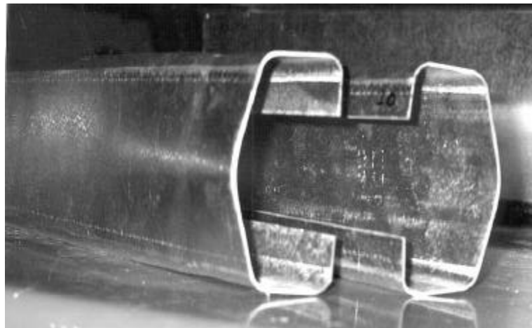
Figure 3.7 End Two Flange Loading, ETF, of C-Sections
