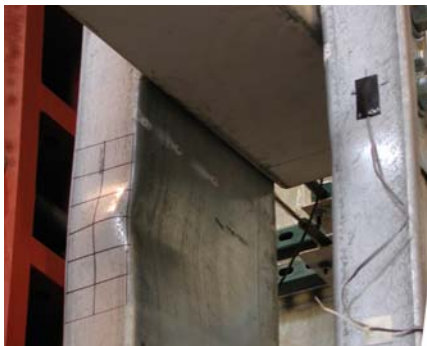
(a) Specimen 2 at 10% Story Drift
