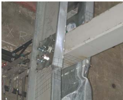
(b) Specimen 4 at 7% Story Drift
